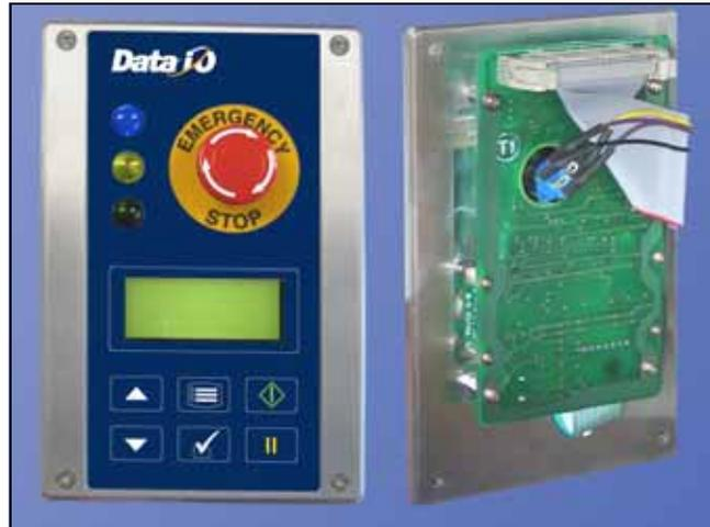
Figure SX-25—Control Panel Module, front and back
