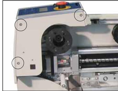
Figure SX-26—Corner Panel Cover with screw locations circled.
