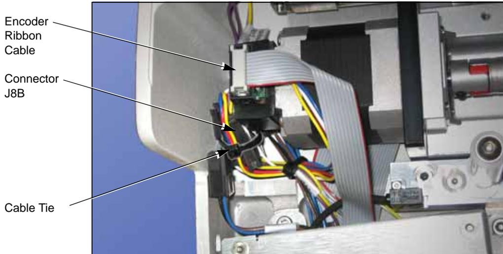
Figure SX-51—Two wire connectors must be unplugged from the Linear Stage Module.
