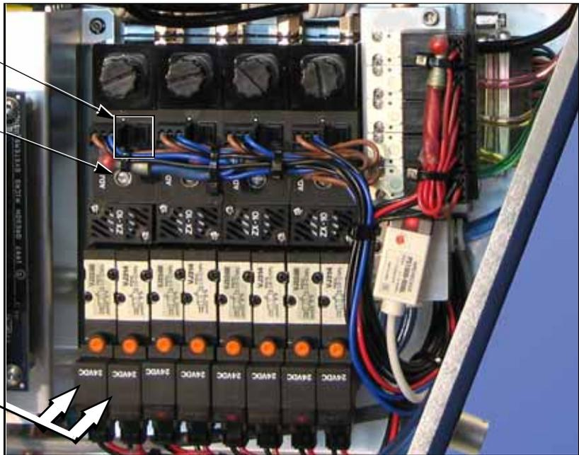
*Figure SX-35—Pneumatic Valve Block. When the vacuum for Probe 1 is enabled, the two small LEDs on the solenoids (white arrows) for Probe 1 will be unlit.*
