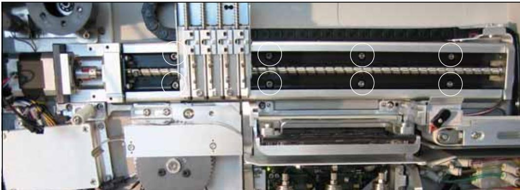
Figure SX-52—Linear Stage Module screw locations (circled). (The Conveyor Module would not be in place at this time.)
