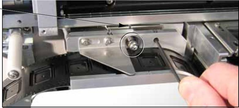
*Figure SX-6—Adjusting the 32/44 mm Tape-In Module: loosening the Centering Bar screw. The Position Locking screw (circled) is already loosened.*
