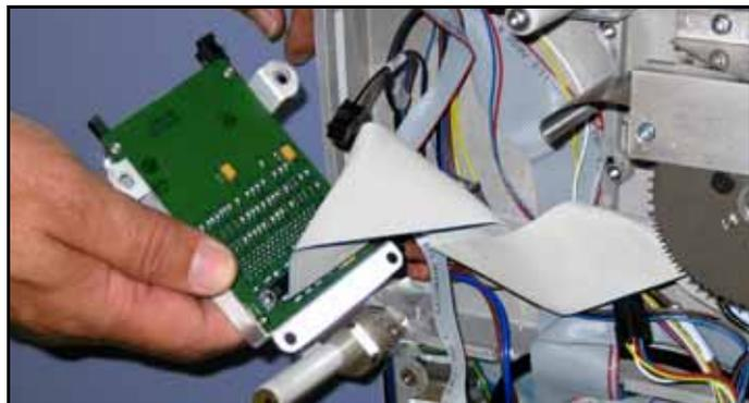
*Figure SX-31—PC Drive Ribbon Cable is attached to the back of the drive.*
