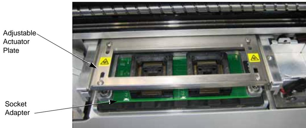
Figure SX-55—Actuator Plate Assembly and Socket Adapter
