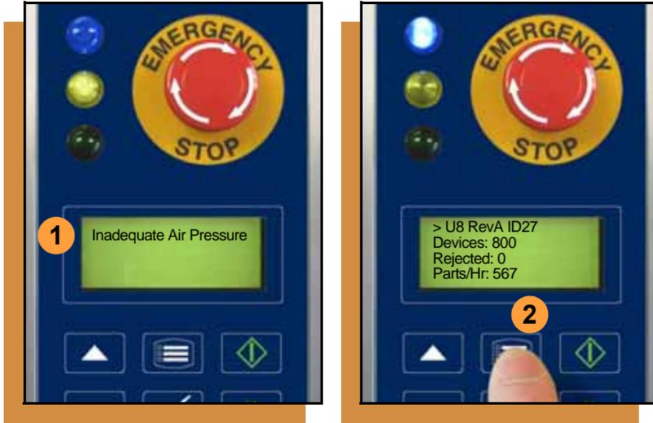
To view and correct errors that appear in the keypad display:
