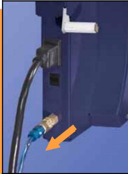
4. Connect to a grounded power source. RoadRunner3 accepts power between 100 and 240 VAC, 50/60 Hz.
