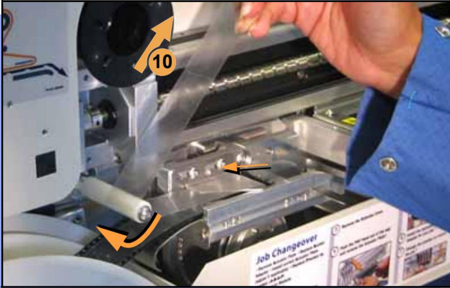
9. Separate the cover tape from the device tape as you advance it.
