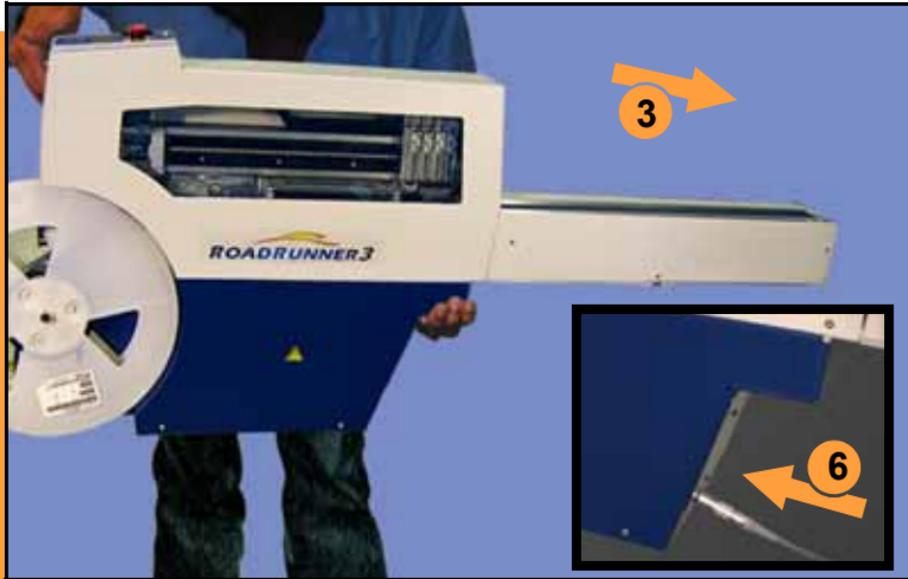
3. Slide the nose of RoadRunner3 under the hook so the teeth engage the pin next to the hook.
