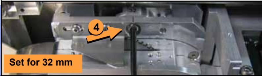
*ROADRUNNER3's* Tape-In Module can be adjusted for 16, 24, 32 and 44 mm device tape widths. A notch points to an etched number indicating the current setting.
