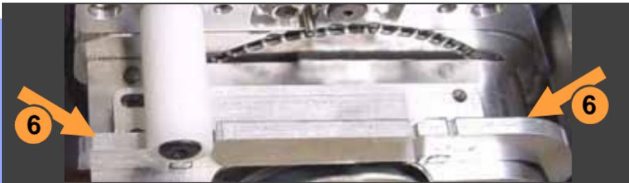
3. Rotate the 3-Position Spacer with your finger until you read 16, 24 or 32, corresponding to your tape width.
