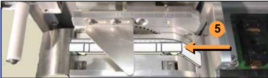
4. Remove the magnetic Front Track for 32 mm (if it is installed) by first, loosening the two Peel Bar screws.
