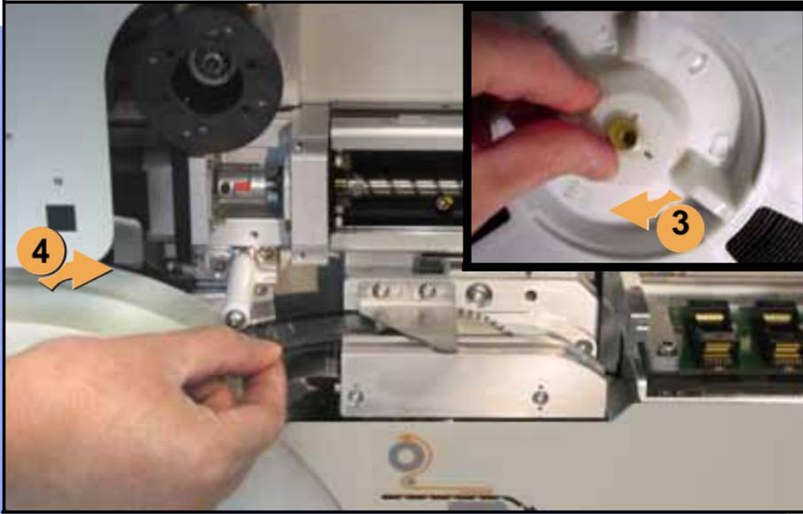
To load and thread device tape:
