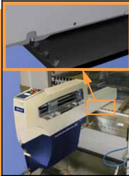
3. Slide RoadRunner under the hook so that its centering teeth engage the pins next to the hook.
