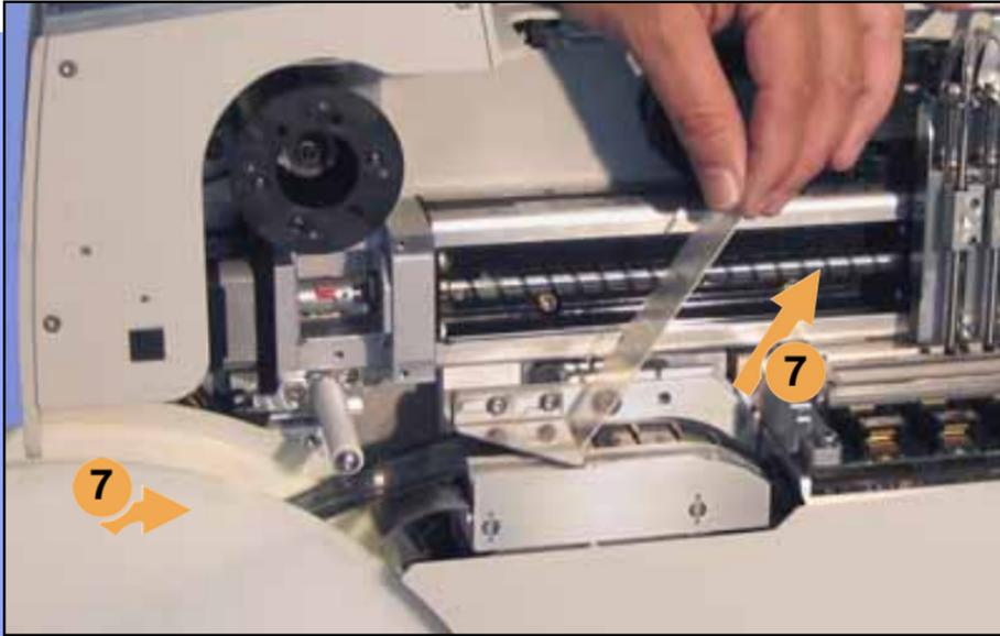
7. Separate the cover tape from the device tape.
