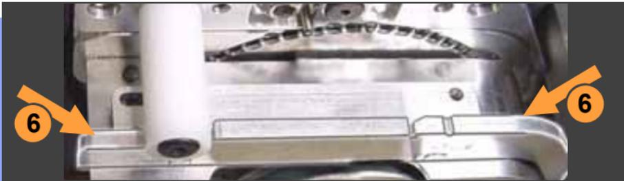
3. Rotate the three-position spacer with your finger until you read 16, 24 or 32, corresponding to your tape width (rotates one direction except when at 16).
