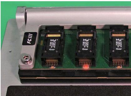
Figure 11: The illuminated LED at socket two indicates that programming has failed.
