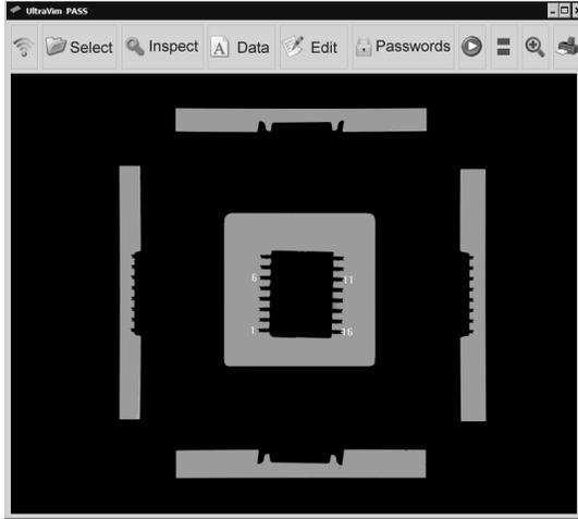
Setting the HideDisplay=2 parameter removes the display on the left side of the screen and all the buttons in the command bar. In this mode the software will start and stop Live Image each time the user clicks on the image.
