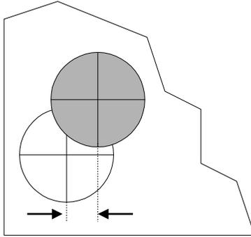
**YTPOS (YTP Error)** is the distance a ball is located from its ideal distance in the Y direction as defined by the edges of the board.
