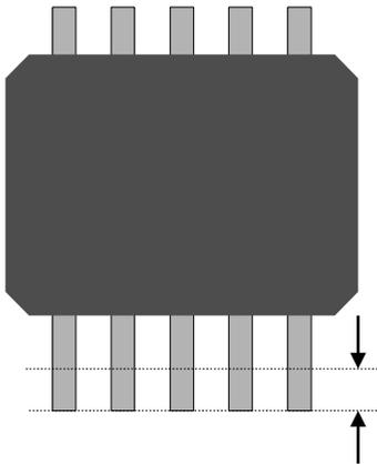
**SLANT (Lead Slant)** is how far the leads on a side are bent in a single direction based on the rotation and alignment of the package body.
