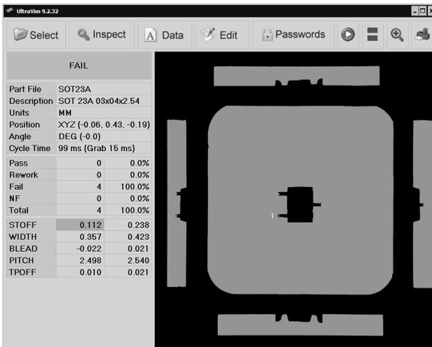
To detect Bent Lead errors more references are needed on the device. To create more references, change the pitch to half of the pitch on the drawing and increase the number of leads from two to three on the first side. Also, add two leads on sides two and four and three leads on side three.
