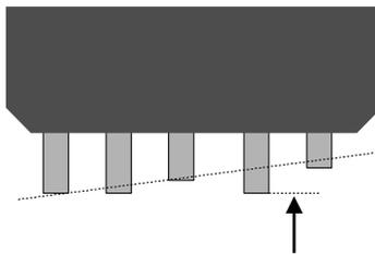
**TPOFF (Tip Offset)** is the distance from the tip of the lead to the ideal position of the lead.
