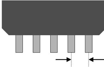
**TPTCH (Total Pitch)** is the distance from the first lead on a side to the last lead on the side.
