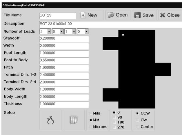
If a 3D inspection is available, select the Standoff FROM PIN measurement instead of Coplanarity. The software will calculate the Standoff of each pin to the part body.
