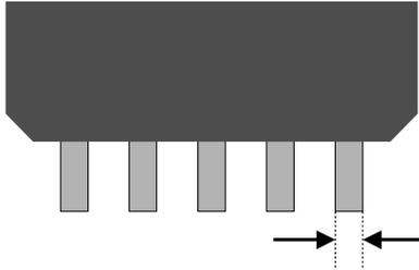
**LSKEW (Skew)** is the absolute value of the bent lead error combined with half the value of the width error. A lead that is bent and has a large width will produce the largest skew error.
