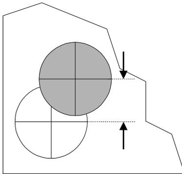
**RTPOS (RTP Error)** is the distance a ball is located from its ideal distance in the XY direction as defined by the edges of the board.
