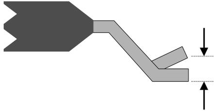
**STOFF (Standoff)** is the distance from the body to a flat surface when the part is placed on that flat surface.
