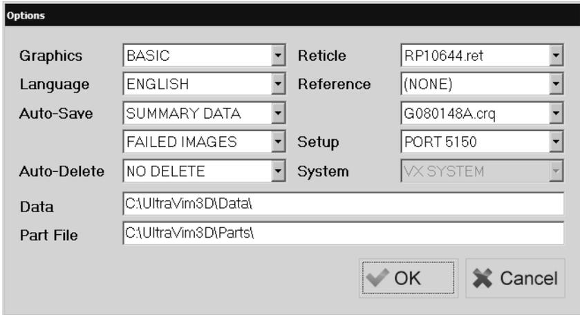
Failed images will be saved in the lot data directory and will start with “PRT” and end “-1.tif” for the first camera and “-2.tif” for the second camera, if the inspection module uses more than one camera. The raw TIF file format is used because it is not compressed which allows the computer to save images faster.
