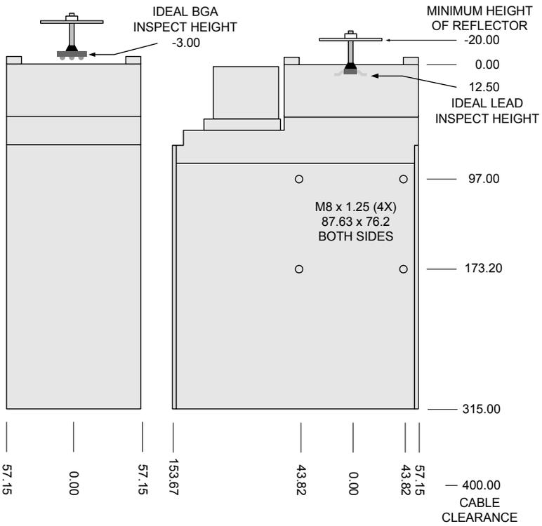
RF4022 © 2013 SCANNERTech LLC. UNITS IN MM.
