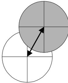
**XTPOS (XTP Error)** is the distance a ball is located from its ideal distance in the X direction as defined by the edges of the board.
