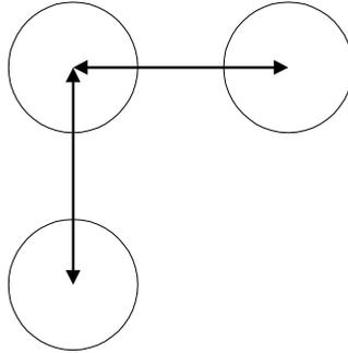
**XPTCH (X Pitch)** is the distance from one ball to the next adjacent ball in the X direction.
