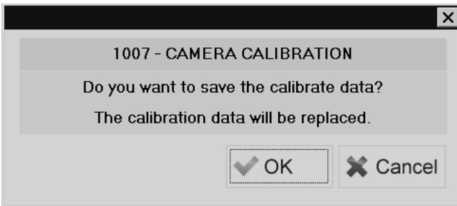
The default calibration for user level 2 is a verification of the calibration. If the calibration was successful the user may save the verified values and the date the verification was completed.
