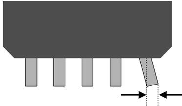
**BLEAD (Bent Lead)** is the distance from the center of the lead to the ideal center of the lead.
