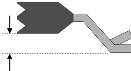
**QWARP (Warpage)** is an estimate of the amount that the part is warped based on a regression of the lead positions.
