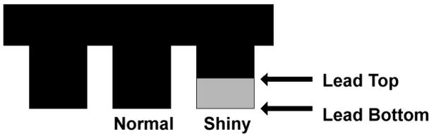
The Shiny selection in the F8 screen allows the user to select software (Shiny SW) or hardware (Shiny HW) compensation. The software compensation will cause the software to automatically adjust the contrast of lead tips. The hardware compensation will cause the software to take two images with opposing side lights turned off if the QFP head is wired to support that. A head wiring with configuration #0 has lights 2,3 on channel one and a head #1 has lights 1,2,3,4 on the first channel.
