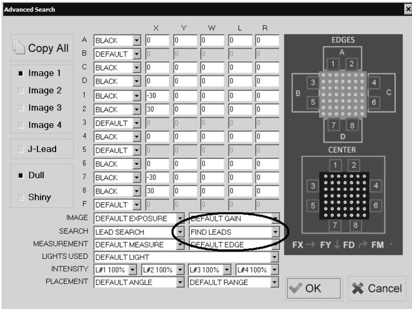
Make sure the SEARCH settings at the bottom of the screen are set to LEAD SEARCH and FIND LEADS. Even though the search is finding the body on side 3 the software considers this a virtual lead that it uses to make calculations.
