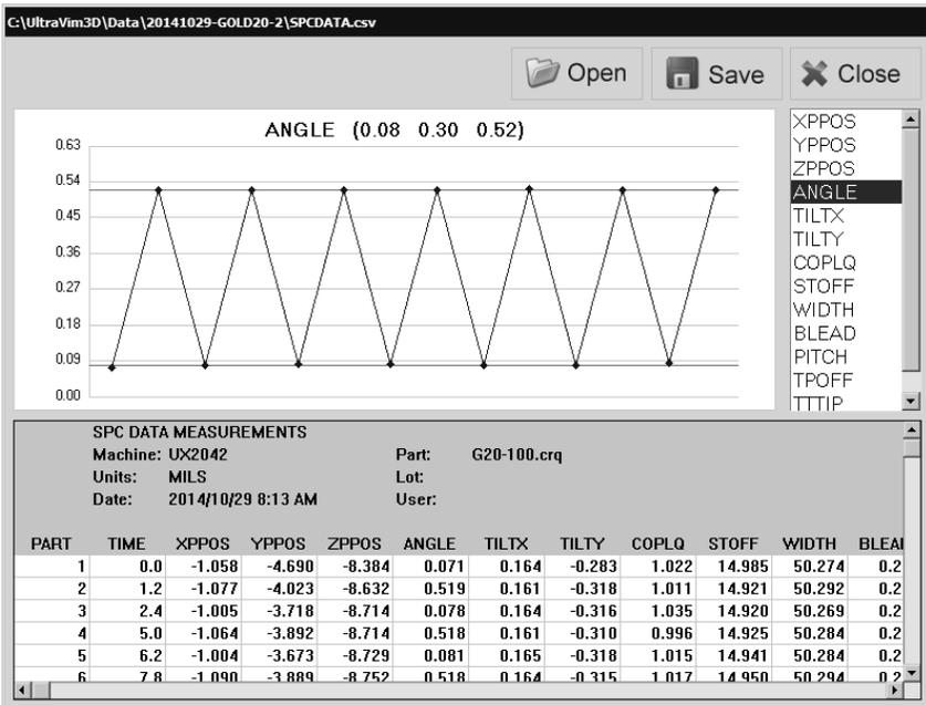
The AutoSaveSPC parameter in the Config.ini file may also be used to save additional data as shown below.
