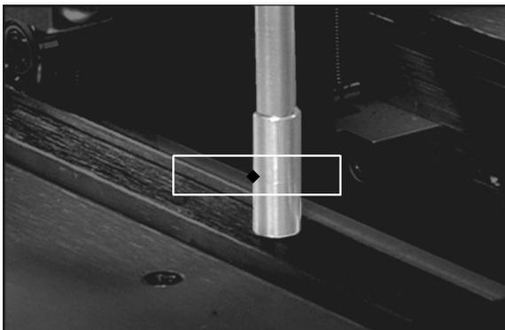
The RIGHT search resulted in +1.1,+0 mm. In the image below, the command “FINDW:-5,-1,5,1,LEFT” was used which resulted in +2.74,+0 mm. The average of the RIGHT and LEFT commands is +1.92 mm.
