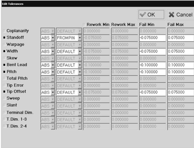
Using the standard part file the software may detect Pitch errors between the first two leads and Standoff errors.
