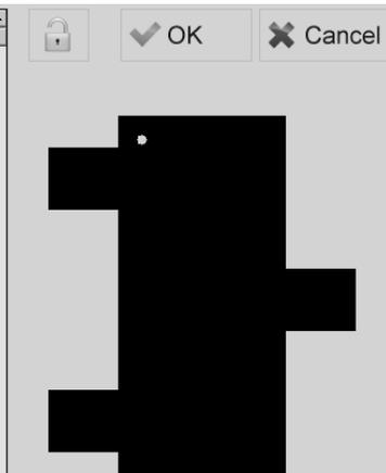
The results of the custom part file are shown below. The third lead has been bent to show that the inspection can detect that failure with the additional virtual leads that use the body of the device as a reference.
