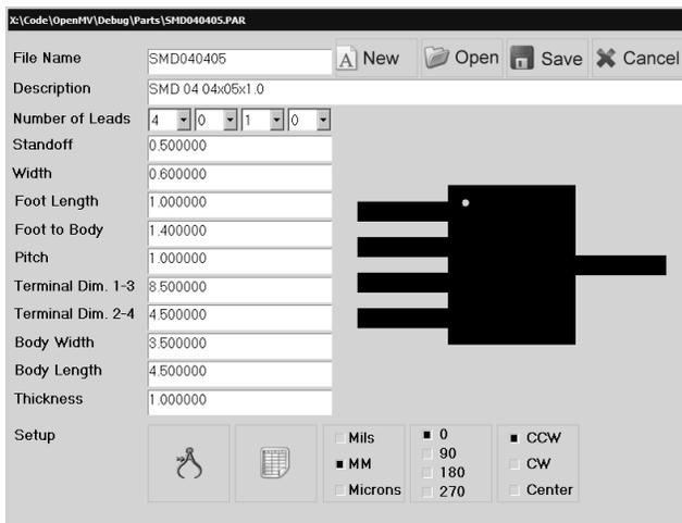
Next click on the spreadsheet icon to define custom lead types and locations. Unlock the spreadsheet and change the label of the fifth lead to B3, the position to half of the body width (1.75) and the type to 213 to define a body reference on side 3. Finally, make the lead width (W) about double the size of the other leads and decrease the length (L) to a smaller number.
