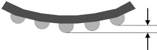
**BHGHT (Ball Height)** is the Z height of the ball relative to the board. This measurement is calculated by adding the nominal standoff to the ball height relative to the closest balls.
