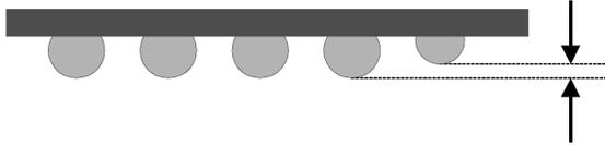
**BWARP (Warpage)** is the estimated Z position of the package substrate at the X, Y position of each ball.
