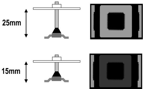
In addition to the GRABT method, the software also has the ability to automatically adjust the gain of the center image. In the example below the center has a background of 20. Setting `AutoGainQfp=1` allows the software to increase the background brightness. Note that this method may cause some inaccuracies on measurements like Width if the contrast is too low. Increasing the gain of an image also increases the noise.
