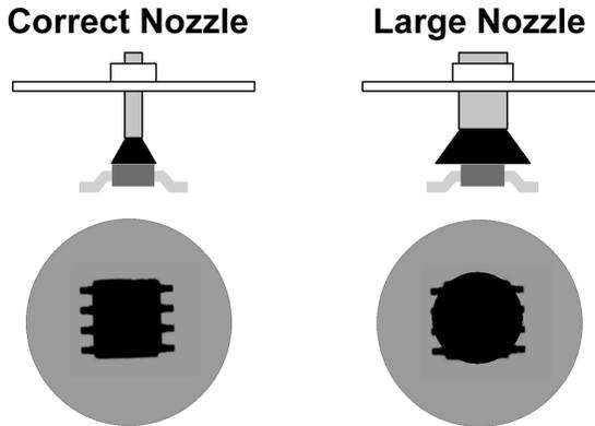
For BGA devices the nozzle may be slightly larger than body of the device if the Body Width and Body Length calculations are changed to CORNER in the Tolerance screen. It is also possible to inspect BGA devices without any background, but changes must be made to the Advanced Settings and some measurements like Body Width and Length will not be available.
