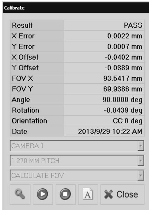
Make sure the optics and pattern are clean and click on the inspection icon to perform a calibration. If the calibration was successful the software will measure several dots and report the placement results as X Error and Y Error. It will also calculate the center of the pattern and the field of view.
