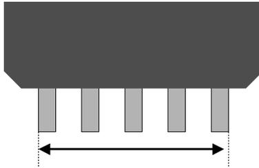
**TPERR (Tip Error)** uses a best-fit line to calculate the tip offset relative to the other leads on a side.
