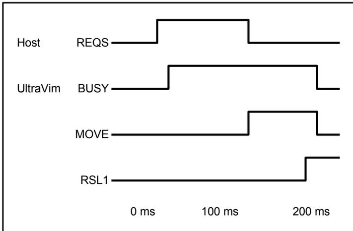
If the inspection result was PASS, both RS1 and RS2 will be set high by the software. If the inspection result was NF (Not Found) or FAIL, both RS1 and RS2 will be set low. If the result was REWORK, RS1 will be high and RS2 will be set low.
