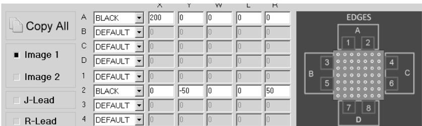
Search F is actually not a search, but instead is a final adjustment to the results calculated from Searches 1 through 8. By changing Search F from DEFAULT to X-Y-D-M-S, you can adjust the final search location in X, Y, degrees, minutes and seconds.
