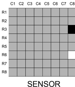
In the example below, a ball is seen as a group of bright pixels. A variety of image processing algorithms such as threshold or edge finding can be used to find the location of the ball center in pixel coordinates. Image processing applications use sub-pixel algorithms that can determine the locations of features to a fraction of a pixel if the image quality is good.
