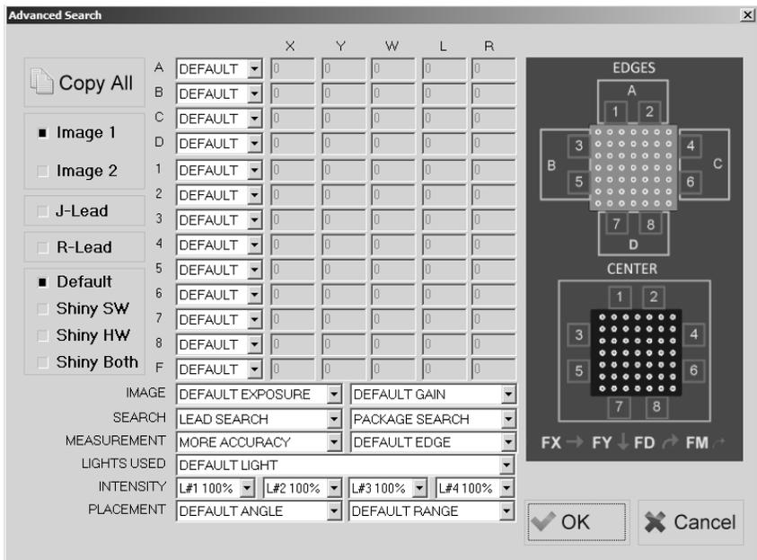
There are two types of rough searches – CENTER and EDGES. The CENTER search determines an automatic threshold and then finds the average location of all pixels above that threshold. This can be useful for leads with front lighting. To force the software to use the CENTER search change Search A from DEFAULT to CENTER.
