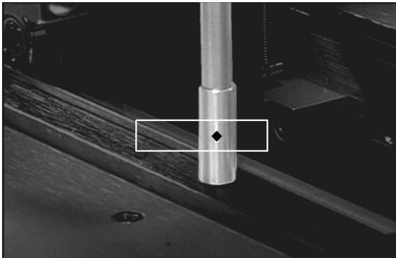
One strategy to with thresholds is to use the result data to adjust the search location and locate the pixels multiple times. Using the original search and the results of +2,-0 mm a new command of “FINDW:-3,-1,7,1” was sent in the example below which again resulted in a location of +2,+0 mm.
