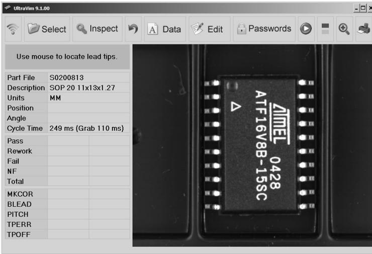
The user must use the mouse with the left mouse button to draw a rectangle from the tip of the first lead to the tip of the last lead. If the software successfully locates the leads, the rectangle will turn green. If the software does not find the leads, the rectangle will turn red.
