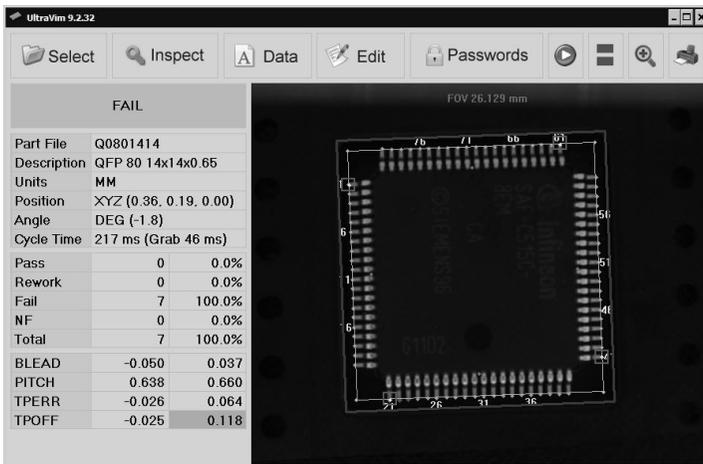
The LOCATE graphics will also show the calculated Field of View (FOV) at the top of the image after an inspection. This calculation is accurate to better than 10% when a known good device with more than ten leads is used. If the calibration is off by more than 10% the FOV text display will be shown in red.
