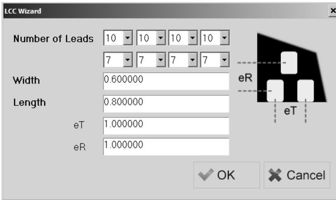
To define a device with a dual set or rows, set the number of leads in the second row of lists and set eR, which is the distance from the first row to the second row of pads as shown in the diagram on the right side of the Wizard dialog.
