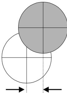
**YPERR (Y Error)** is the distance a ball is located from its ideal distance in the Y direction.
