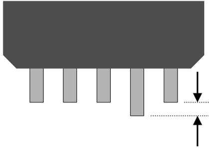
**SWEEP (Lead Sweep)** is how far the leads are swept in the tip offset direction as defined by the location of the package body.
