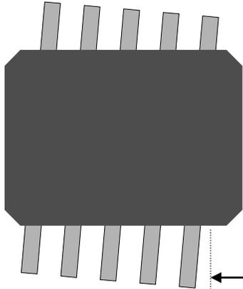
**TTTIP (Terminal Dimension)** is the tip-to-tip distance between two opposite leads.
