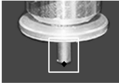
In the example below, the command “FINDW:1.3,-4.5,2.2,-3.4,UP” was used. In this example, the FINDW command was successful because the search box was smaller and did not include the upper white part of the round ring.
