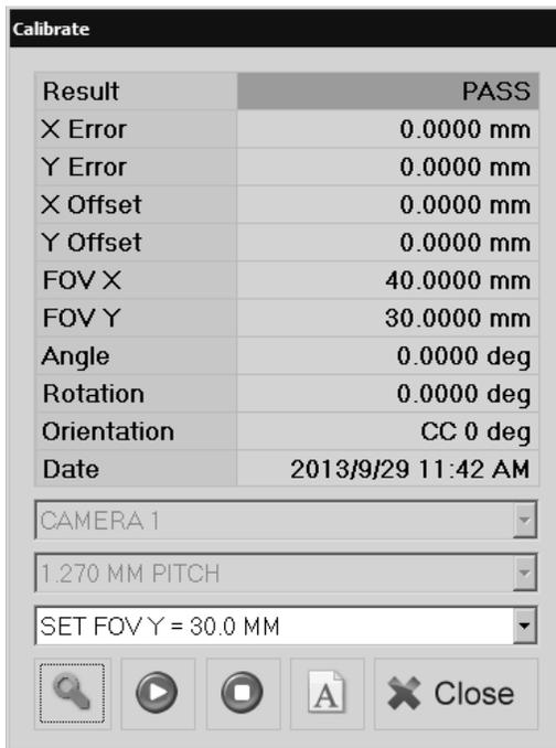
The software will only simulate cameras that are perfectly orthogonal to the view. This can be useful for 2D applications, like 2D lead inspection, where you may not have a calibration target but still would like to estimate world units in the image. Note that the calculated field of view will be shown with debug graphics when you successfully inspect a leaded part. This can be a useful method
