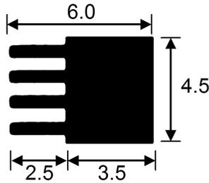
To create the part file, enter all the dimensions off the drawing but add an additional lead on the third side and calculate what the terminal dimension would be with leads on the third side, which is 8.5 in the example below. These dimensions will act as a reference point that will allow the software to make calculations.
