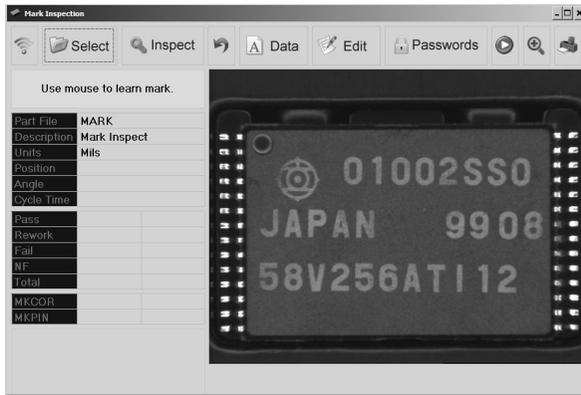
The size of the graph and results on the left of the screen can be changed using the DefaultGraphCX parameter, which must be at least 300 pixels wide. Setting HideDisplay=1 will remove the displays on the left side of the screen.
