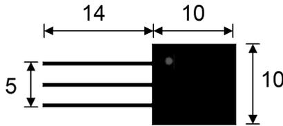
To create the part file, enter all the dimensions from the drawing but calculate what the terminal dimension would be with leads on the third side. These dimensions will create reference points that will allow the software to make calculations.
