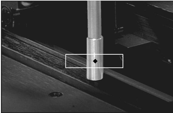
The FIND commands may also be used with the directions UP, DOWN, LEFT or RIGHT to find edges. In the image below, the command “FINDW:-5,-1,5,1,RIGHT” was used.
