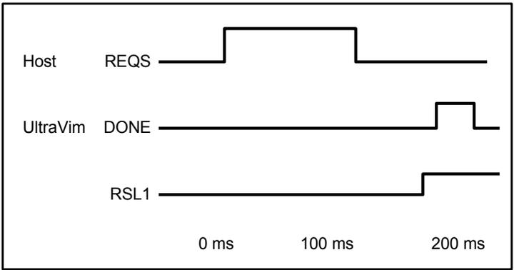
The diagram below shows the timing when UseDoneSignal=1 is set in the Config.ini file and the DIGITAL PF configuration is selected. In this case the PASS or FAIL line will act as a signal to let the host know when inspection is complete.
