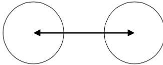
**YPTCH (Y Pitch)** is the distance from one ball to the next adjacent ball in the Y direction.
