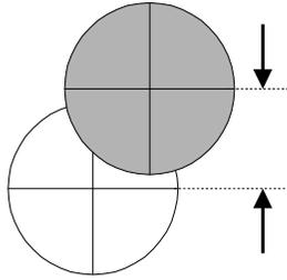
**RPERR (R Error)** is the distance from the X,Y center of the ball to the ideal X,Y center defined by the X and Y datum.
