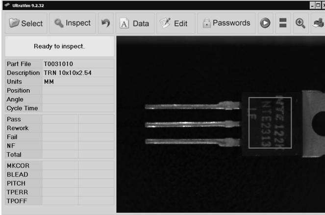
With the LOCATE graphics on you can see the light blue search box that locates the leads of the part. The size of this box can be controlled with the Foot Length setting. In the example below the Foot Length has been set to 5.
