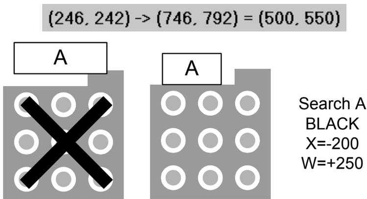
However, more adjustments are required for this irregular device before we are ready to inspect. Searches 1 to 8 are used to calculate the fine location of the device. Search 2 must be adjusted so the software knows where to find the irregular feature on the device. This can be done by setting the search to BLACK, setting Y to -50 and setting R to +50.
