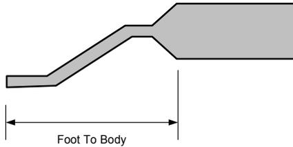
Standoff is calculated from the triangulation of the intersection of the rays shown in the diagram below. Rays 1, 2, 3, and 4 can be calculated from the information in the views, but ray X cannot be found because of the lighting configuration. To compensate for this, the software creates a “Virtual Ray X” during the inspection from the “Foot to Body” dimension.
