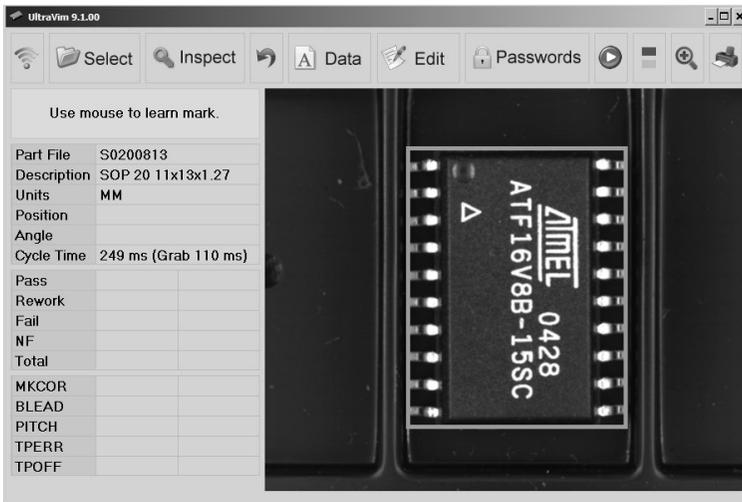
With LOCATE graphics on a light blue search box will appear on each side around the leads. The size of the search box can be changed with the Foot Length parameter in the part file.
