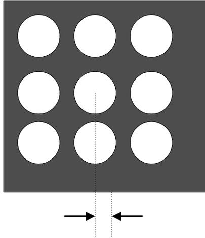
**GYOFF (Y Grid Offset)** is the Y offset of the center of the ball array grid to the center of the package.
