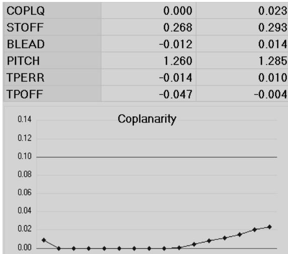
To display other measurements use the mouse to click on each item above the chart. For example, below the user has clicked on TPOFF to display the Tip Offset results. Note that the failure tolerance settings are displayed in the chart with red lines.
