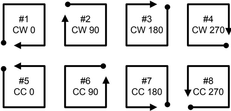
The orientation values stored in the Config.ini file for an UltraVim UX module are shown below.
