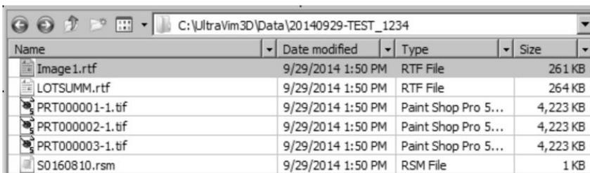
Failed images will be saved in the lot data directory and will start with “PRT” and end “-1.tif” for the first camera and “-2.tif” for the second camera, if the inspection module uses more than one camera. The raw TIF file format is used because it is not compressed which allows the computer to save faster.
