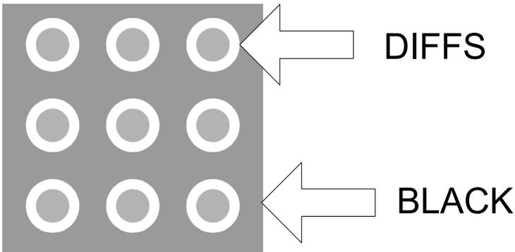
The diagram below illustrates finding a WHITE edge where the leads are front-lit and the background is black. Using a DIFFS search would also find the leads because the black space between the leads creates differences in the image.
