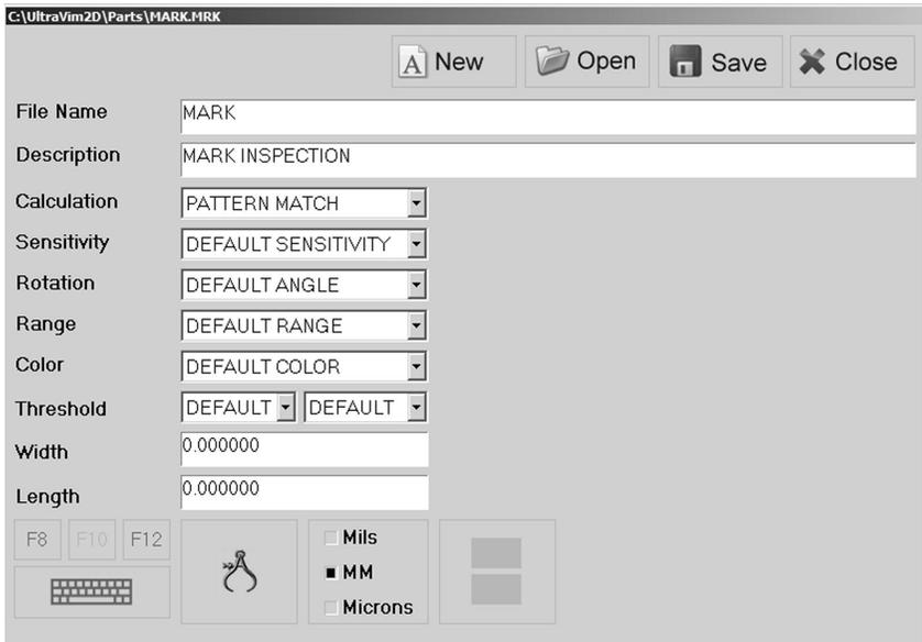
**Calculation** is set to PATTERN MATCH, which is normalized grayscale correlation. The SPLIT MARK setting will split a mark into smaller segments for more sensitive detection.
