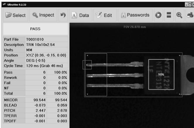
In some cases you may wish to have a larger search box. This can be accomplished by increasing the foot length. Changing SEARCH to PATTERN MATCH in the Advanced Alt-F8 screen will cause the software to search for the entire device as shown below. Note that this method may not be reliable if the mark on the part is changing position or is a label.
