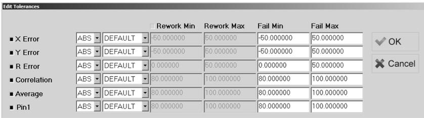
**XPERR (X Error)** is the pixel distance a search is located from its learned position in the X direction.
