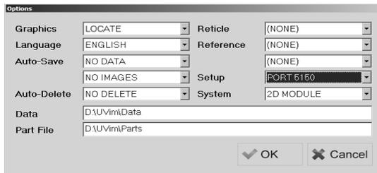
To set the software in a socket server mode, select a port in the Options dialog as shown below. Available ports include 5150, 5151, 5152 and 5153. Other systems should connect to the socket using the computer name that is shown in the passwords dialog or the actual IP address.
