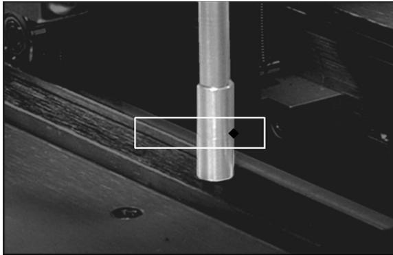
In the image below, the command “FINDW:-1,-8,5,0,UP” was used which returned a location of +2.0,-2.8 mm. Note that coordinate system depends on the camera orientation in the calibration screen.
