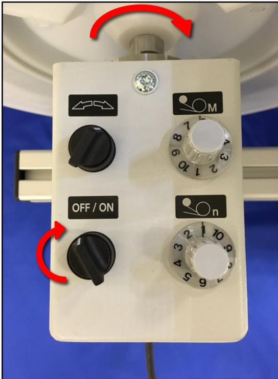
Confirm unit is rotating the spindle.
