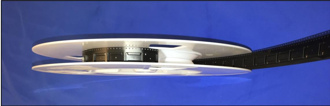
**Connect carrier tape to empty tape reel.**
