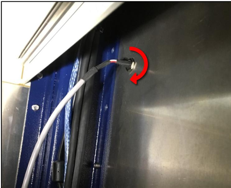
**Fasten Tape Rewind electrical port to side panel/wall.**
