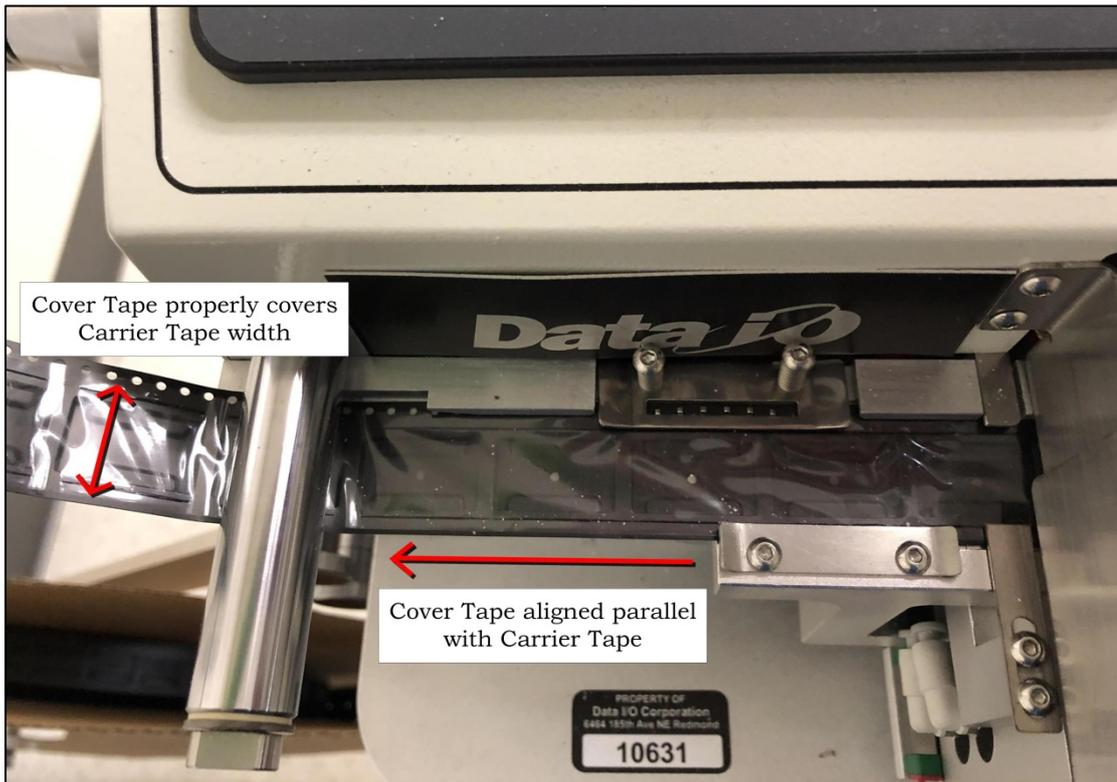
Cover Tape aligned with Carrier Tape
