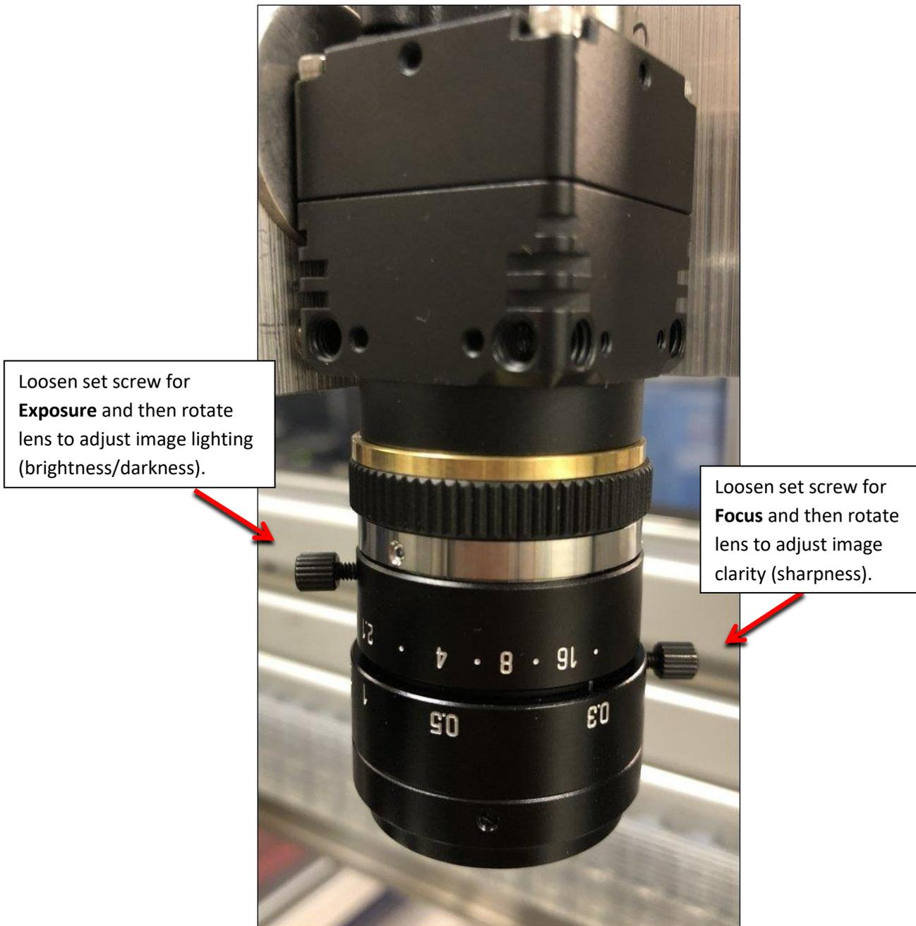
12. Tighten the set screw(s) after adjusting exposure/focus.
