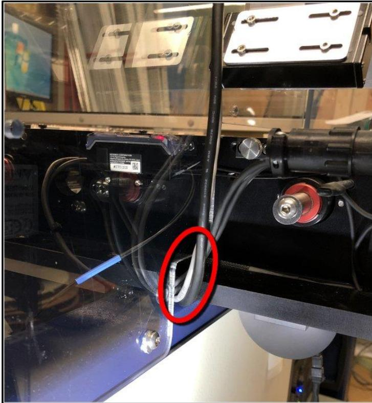
4. In the workspace interior, route the cables toward the rear corner along the base of the blue chassis beam, down into the chassis opening/cut-out in the corner, and into the UltraVIM computer.
