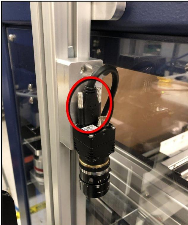
3. Route the other end of the camera cable down, loosely pair it together with the LED Light cable, and route both cables down under the taper and into the workspace (through the clear panel opening).
