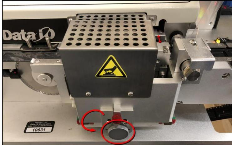
**Figure 27: Adjusting the press sealer/roller position.**
