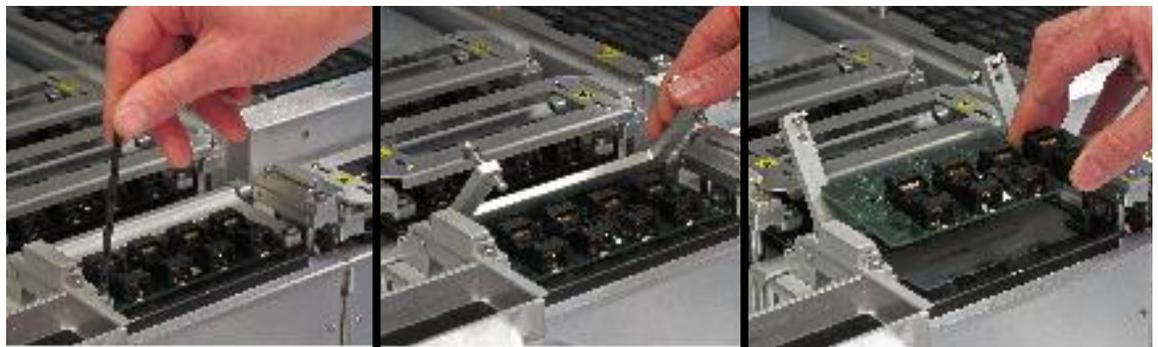
**Figure 32:** Removing the Socket Adapter from a programmer.
