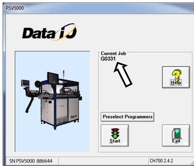
**Figure 60: The CH700 Main window for the PSV5000 opens with a job loaded and job name displayed (arrow).**
