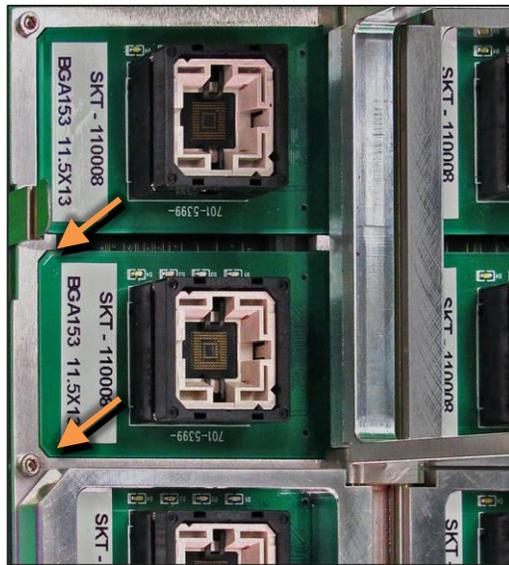
**Figure 36: One clamp open with a Socket Adapter installed. The chamfered corners are to the left (arrows). There is an alignment hole in each corner (two are covered by the label in this view.)**
