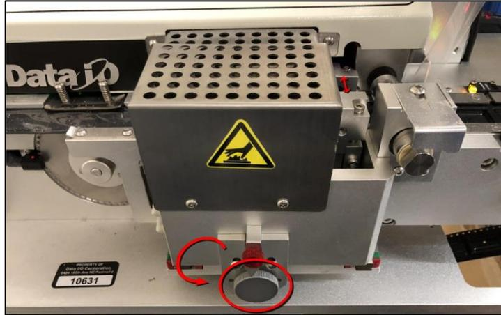
**Figure 22: Adjusting the outer heat shoe position.**
