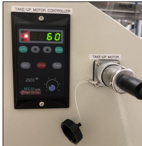
**Figure 18: Press 'Up' and 'Down' arrow buttons for motor tension.**
