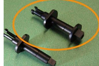
**Figure 40: Different-sized probe tips.**
