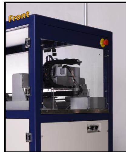
Figure 70: There are two Emergency Stop (E-Stop) buttons: on left near front, and on right near back of the machine
