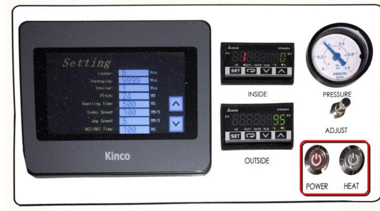
Figure 25: Ensuring the 'Heat' button is OFF.
