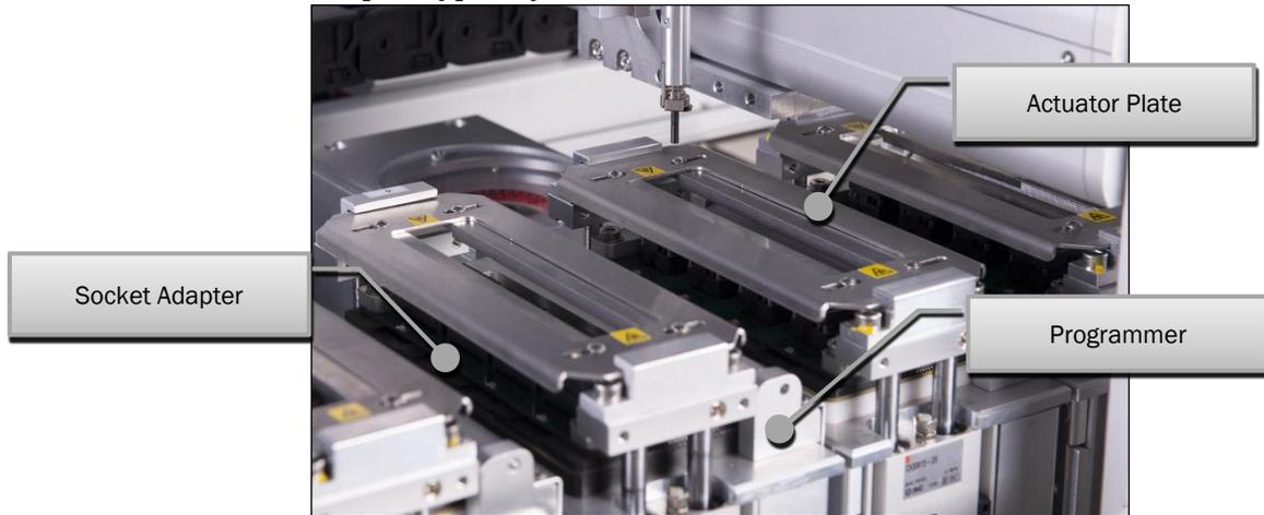
**Figure 6:** FlashCORE III programmers on PSV5000.
