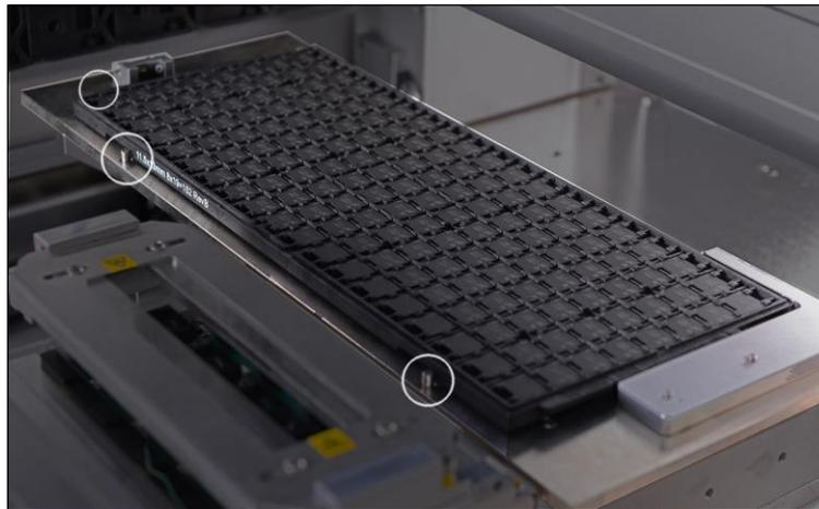
**Figure 5:** To install a tray, index it along the pins (circles). The chamfered corner for the *input* and *output* trays is at the far left corner. *Input* tray position shown.
