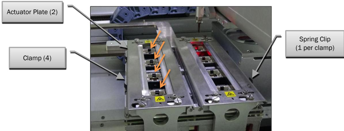
**Figure 4:** One LumenX programmer with eight Sockets held down by four clamps actuated by two adjustable Actuator Plates. Orange arrows indicate Socket Adapters for the front half of the programmer.
