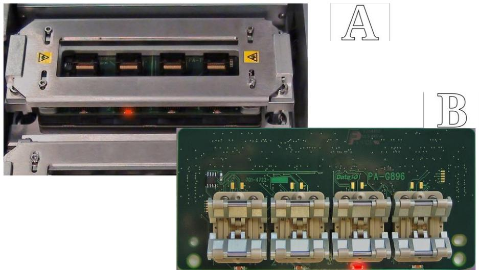
**Figure 7:** Each FlashCORE Socket Adapter has one red LED per socket. A) Standard Adapter; socket 2 has failed. B) HIC Adapter. Socket 3 has failed. The Actuator Plate is not shown on the HIC Adapter for clarity.
