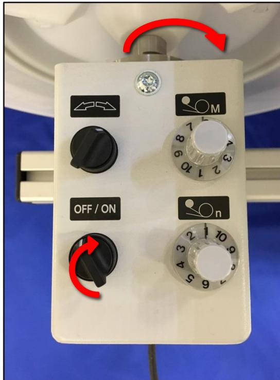
Figure 11: The Tape Rewind motor controls.
