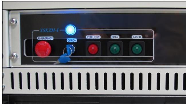
**Figure 74: Laser Control Panel**
