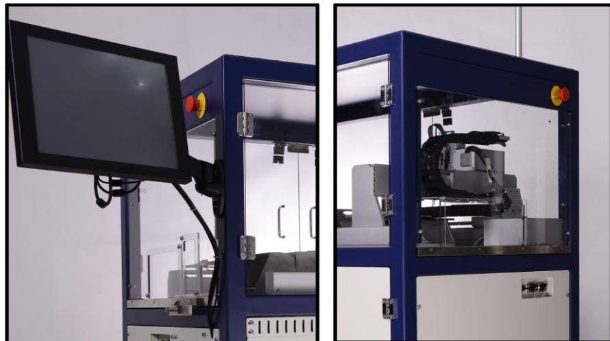
**Figure 2:** There are two Emergency Stop (E-Stop) buttons: on left near front, and on right near back of the machine.
