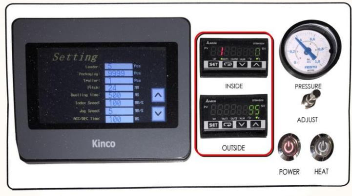
Figure 19: Temperature controls for heat sealer.
