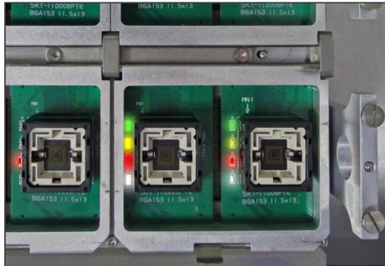
**Figure 5:** Each LumenX Socket Adapter has four LEDs and indicates PIN 1 as shown. All four LEDs light at once only during startup and go off when the startup procedure is complete. The Actuator Plate is not shown here for clarity.
