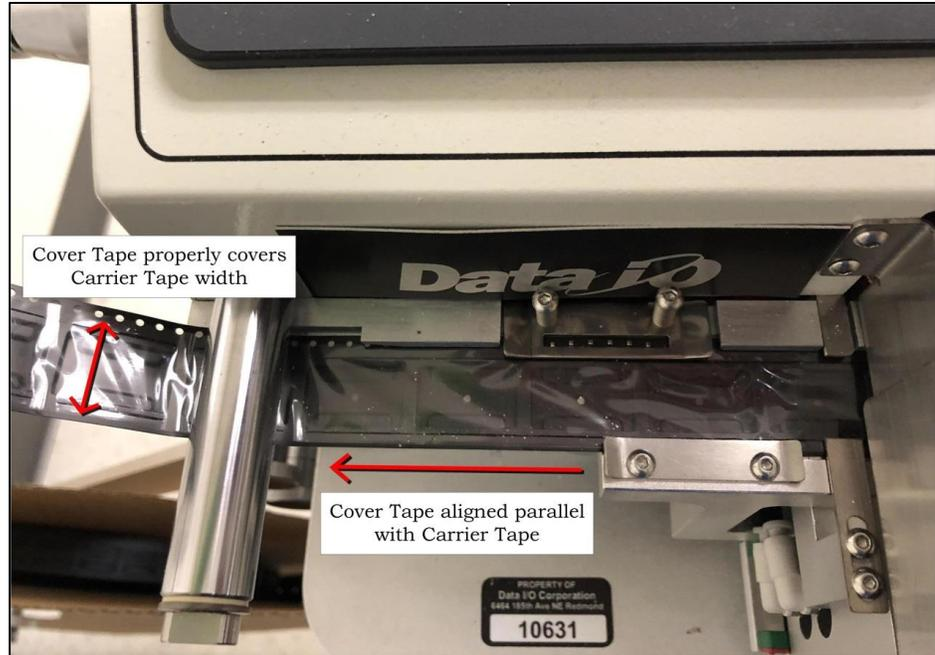
**Figure 17: Align cover tape parallel with the carrier tape.**
