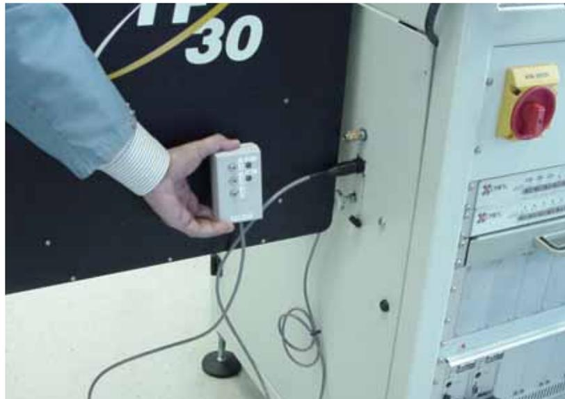
*Figure 1-41—Plug in TF Simulator*
