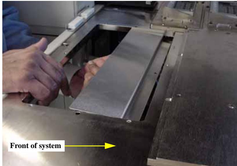
*Figure 1-26—Installing the bottom cover*
