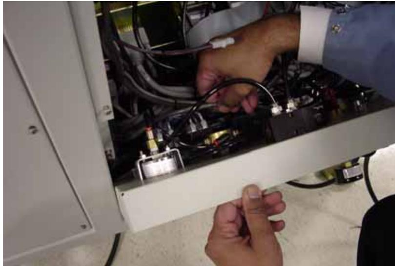
*Figure 1-51—Route wire harness along floor of system*
