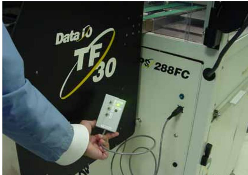
*Figure 1-71—Plug in TF Simulator*
