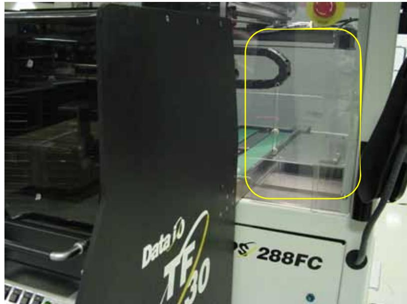
Figure 1-67—Unused slider is closed
