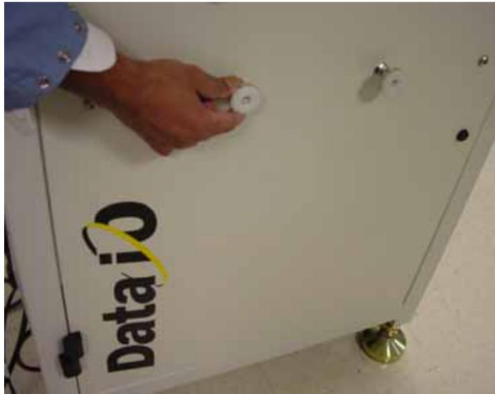
*Figure 1-62—Adjust TF30 supports fully inboard*
