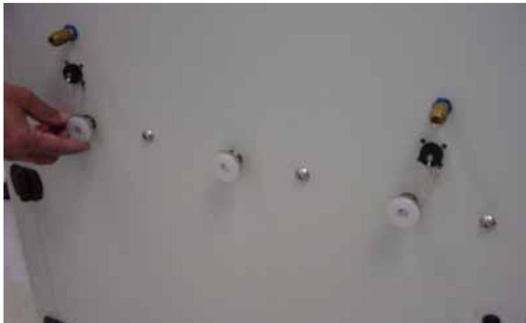
*Figure 1-29—Adjust TF30 supports fully inboard*
