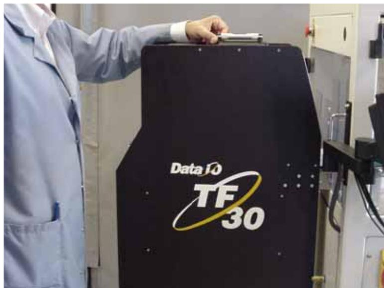
Figure 1-68—Place level on TF30 Tray Feeder
