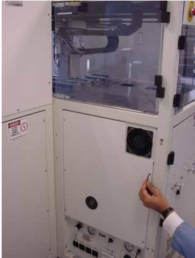
*Figure 1-6—Remove back panel (shown with Option Bay)*
