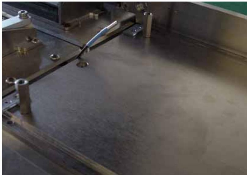
*Figure 1-37—Route fiber optic through access hole*
