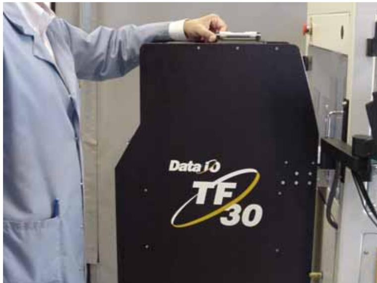
*Figure 1-33—Place level on TF30 Tray Feeder*
