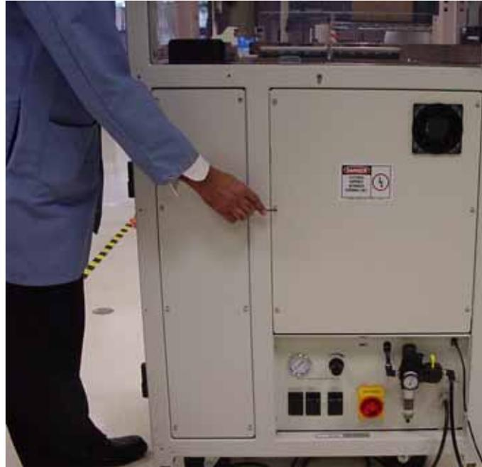
*Figure 1-43—Loosen screws on back panel*
