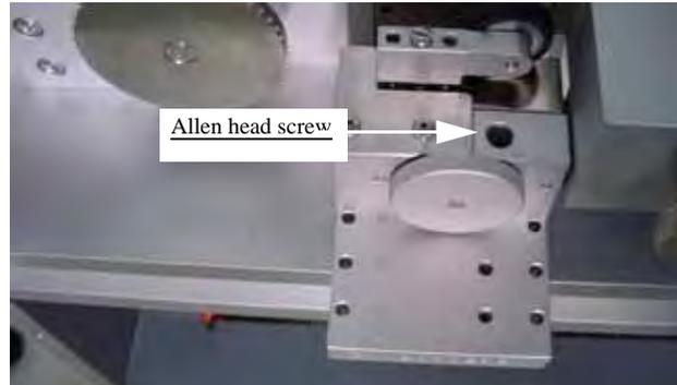
*Figure 2-23—Adjusting width of pressure seal unit*
