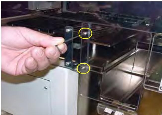
Figure 2-13—Remove two screws holding small safety shield
