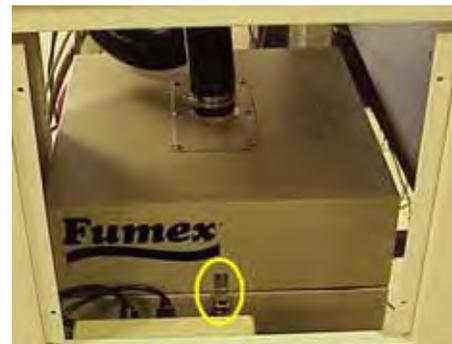
Figure 5-28—Filter system spring clip
