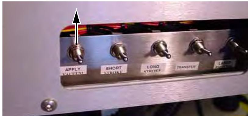
Figure 5-34—Apply Vacuum switch UP
