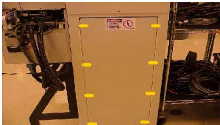
*Figure 5-25—Lower back laser housing panel screw locations*
