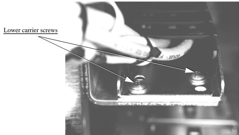
Figure 5-13—Lower carrier screw locations
