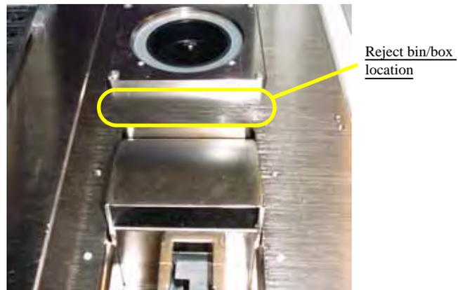
Figure 2-6—Reject bin/box location
