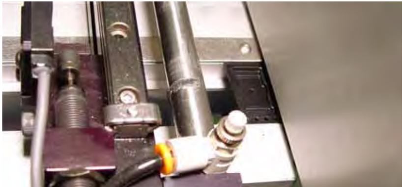
*Figure 2-19—Carrier tape threaded into track*
