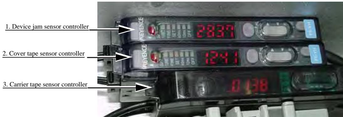
Figure 5-78—Sensor controllers
