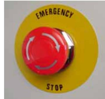
Figure 3-17—Emergency stop (E-Stop) button
