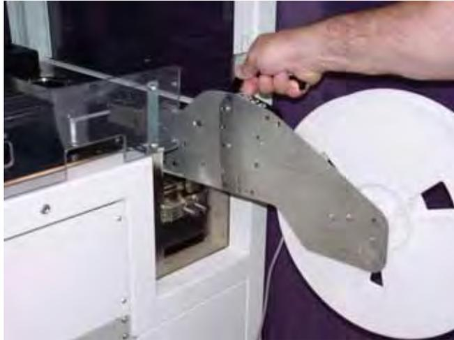
Figure 2-14— Slide feeder unit down channel
