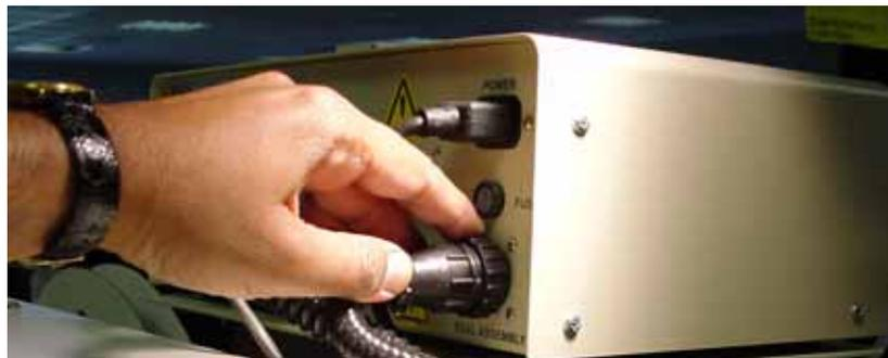
*Figure 2-25—Power cord in tape output controller*
