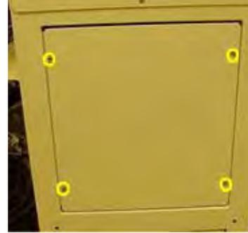
Figure 5-26—Side laser housing panel screw locations
