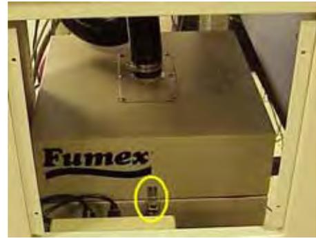
*Figure 5-19—Filter system spring clip*
