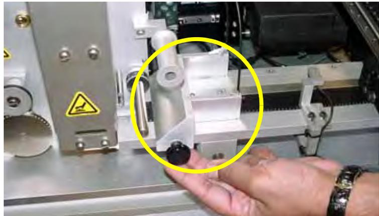
*Figure 2-29—Remove sensor clamp block*
