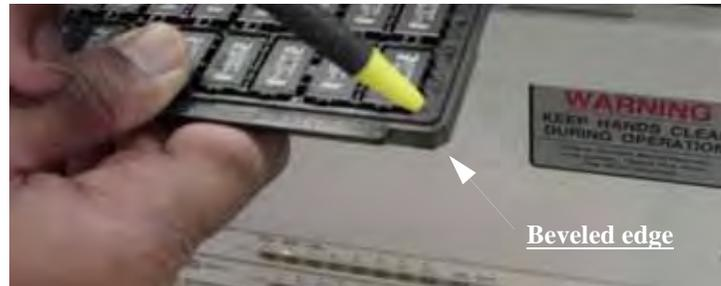
*Figure 2-4—Static tray orientation*
