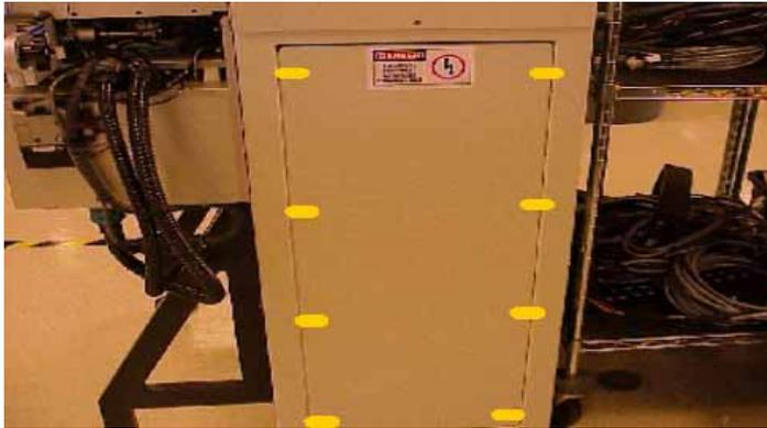
*Figure 5-16—Lower back laser housing panel screw locations*
