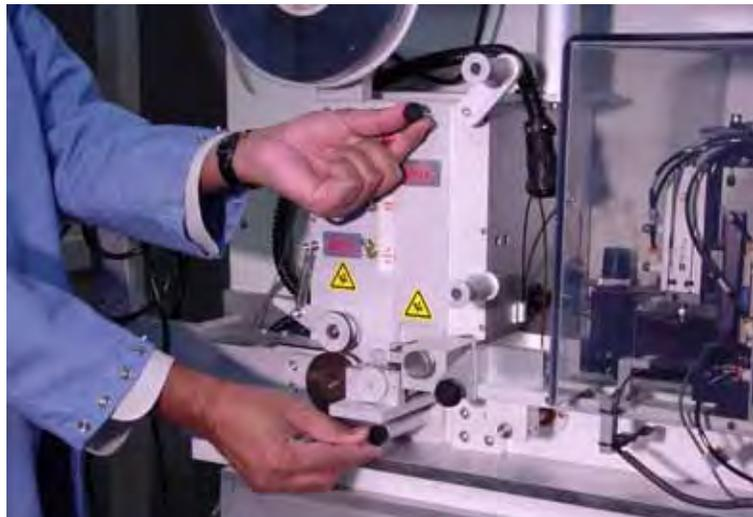
*Figure 2-24—Installing pressure seal unit*
