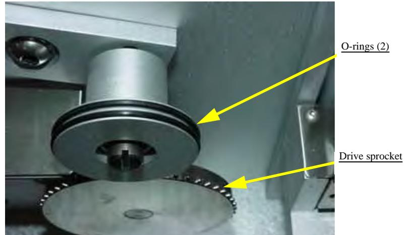
Figure 5-77—Idler pressure wheel and O-rings
