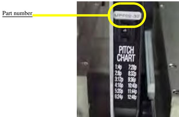
*Figure 2-11—Part number for 32 mm feeder*
