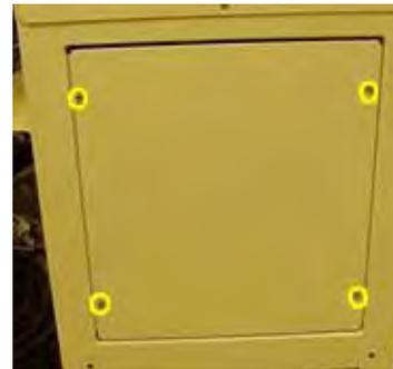
*Figure 5-17—Side laser housing panel screw locations*
