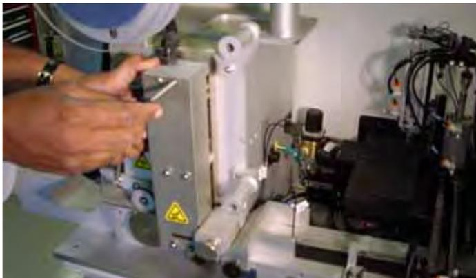
Figure 2-22—Installing heat seal unit
