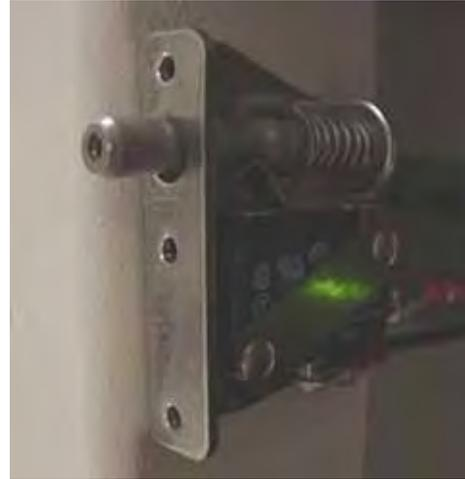
*Figure 1-12—Laser safety interlock*
