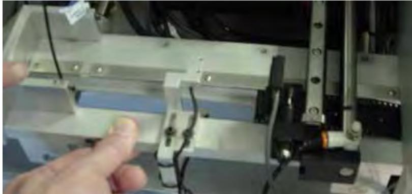
Figure 2-20—Adjustable Loading Track
