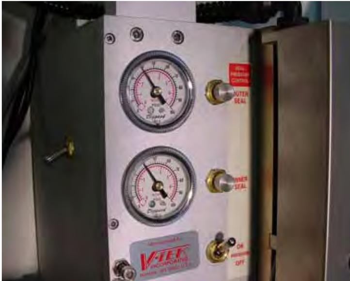
*Figure 2-26—Seal pressure control settings*
