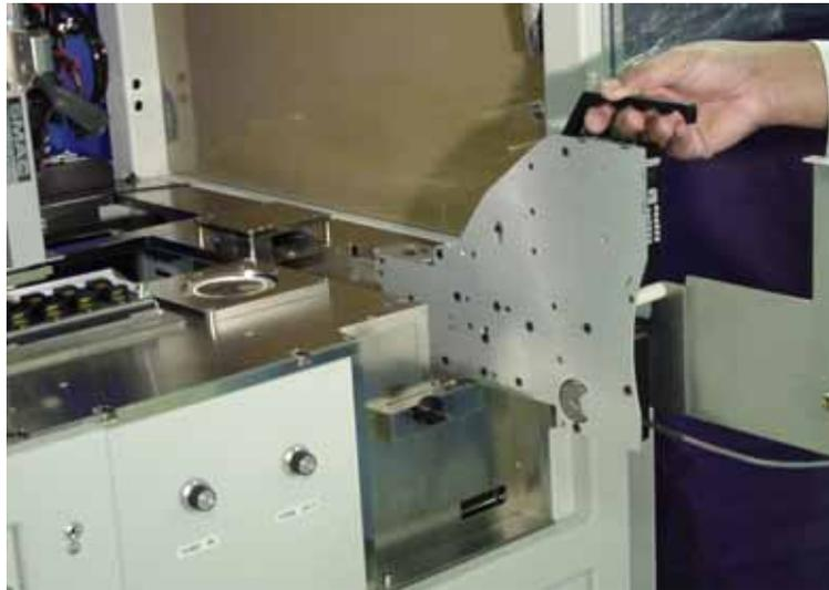
Figure 2-12— Slide feeder unit onto base plate
