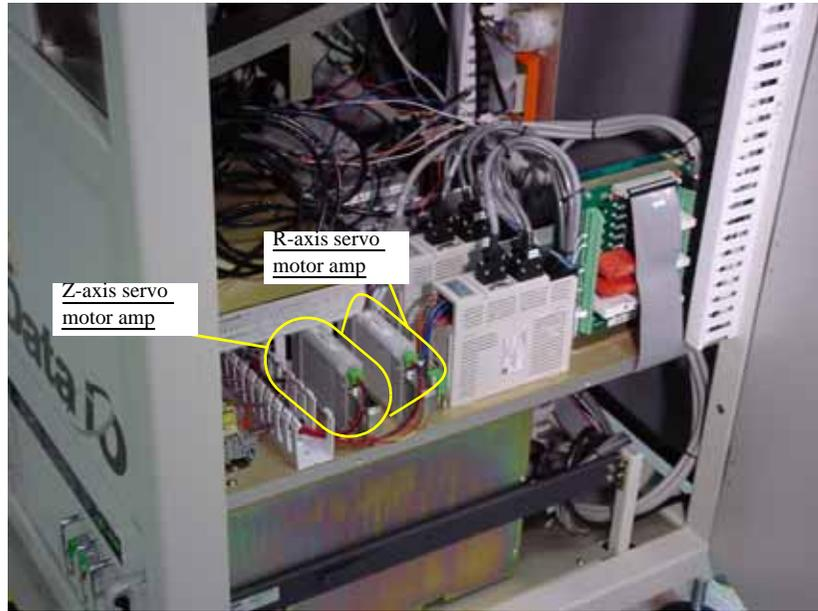
Figure 6-8—Z-axis and R-axis servo motor amps
