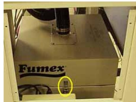
Figure 6-21—Filter system spring clip
