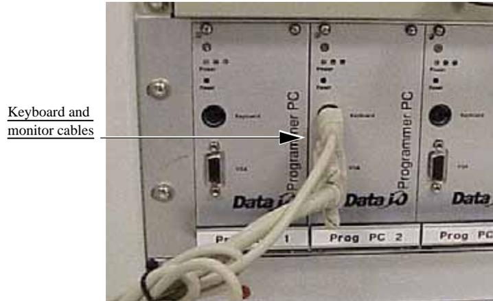
Figure 6-32—Old style KVM with cables
