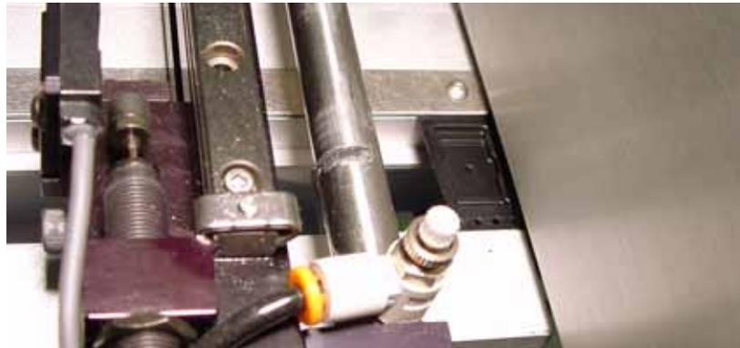
*Figure 2-19—Carrier tape threaded into track*
