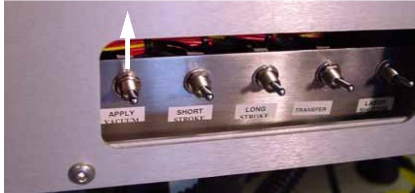
*Figure 6-44—Apply Vacuum switch UP*
