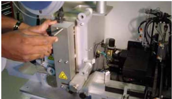
Figure 2-22—Installing heat seal unit
