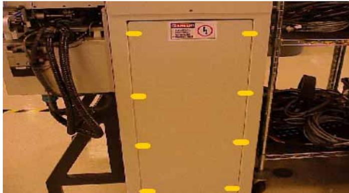
*Figure 6-18—Lower back laser housing panel screw locations*
