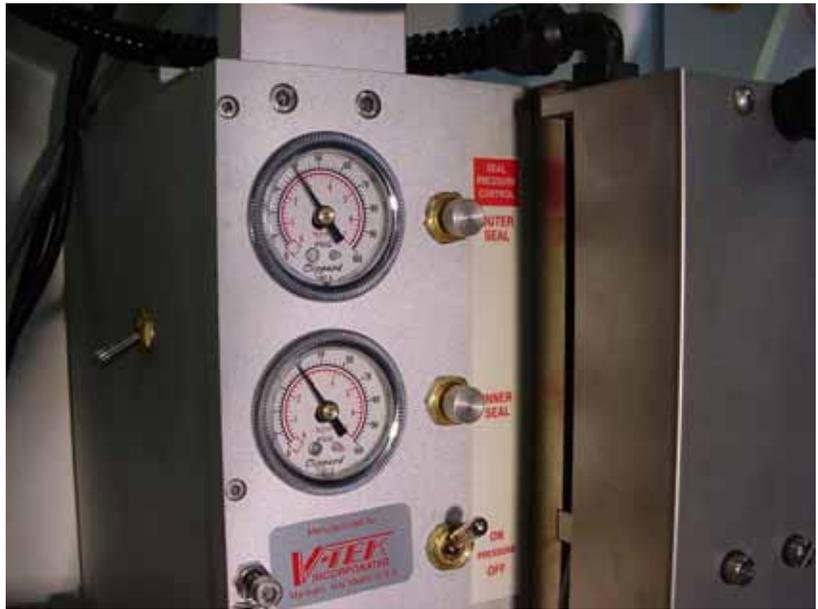
Figure 2-26—Seal pressure control settings
