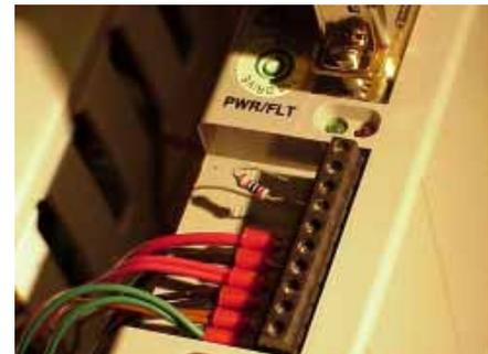
*Figure 6-109—Install resistor***6. Test shuttle transfer assembly—**
