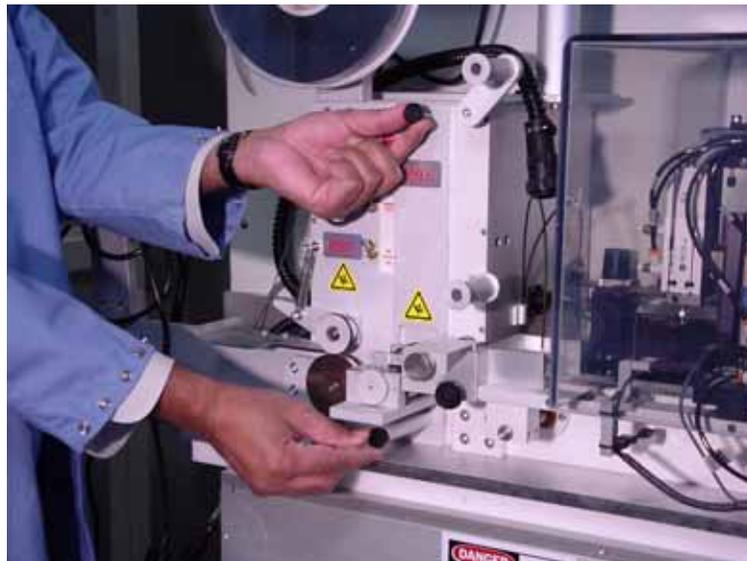
*Figure 2-24—Installing pressure seal unit*
