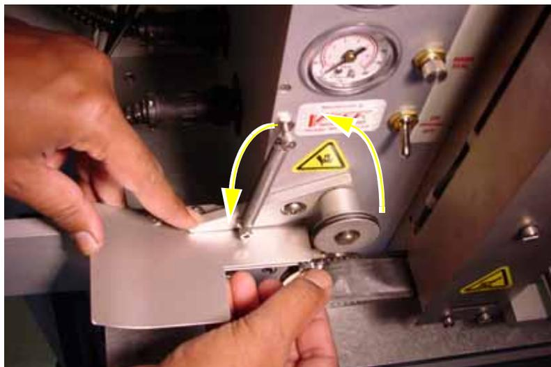
*Figure 2-32—Idler Arm and Drive Sprocket*
