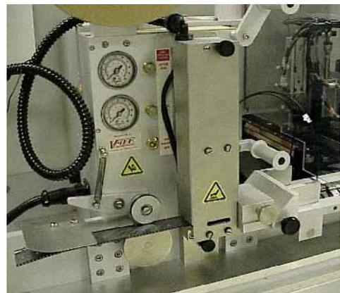
*Figure 2-17—Heat seal unit*
