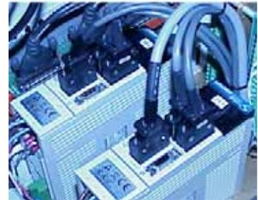
*Figure 6-94—Mitsubishi servo motor amps*
