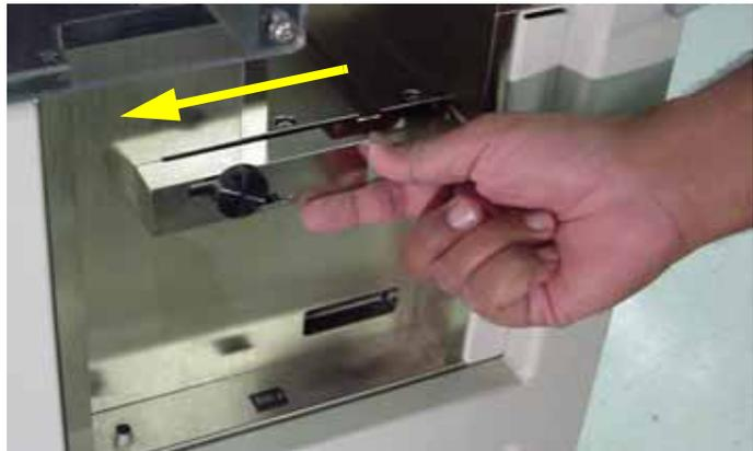
Figure 2-11—Slide lock bar to left
