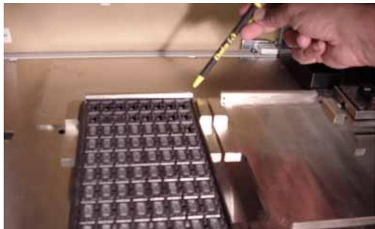
Figure 2-3—Tray seated with optic sensor blocked
