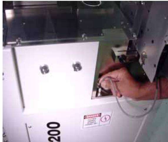
Figure 2-15—Connect interface cable
