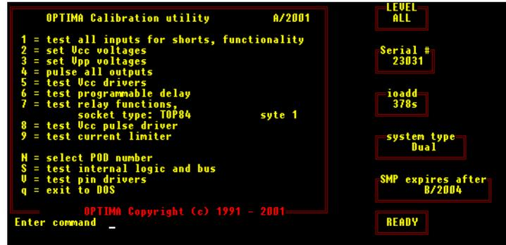
Figure 6-56—Press 2 to set Vcc voltages
