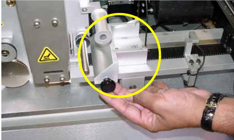
Figure 2-29—Remove sensor clamp block
