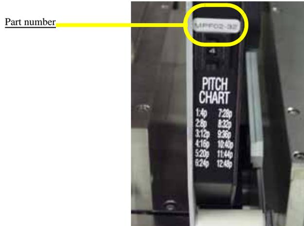
Figure 2-9—Part number for 32mm feeder
