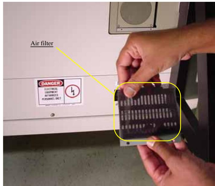
*Figure 6-24—Replace air filter*
