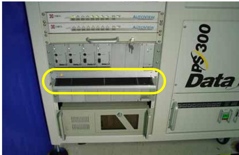
*Figure 6-2—Fan filter drawer*
