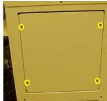
Figure 6-28—Side laser housing panel screw locations
