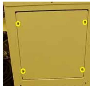
*Figure 6-19—Side laser housing panel screw locations*
