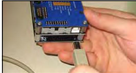
Figure 2-1—Plug the USB Cable into **IW**
