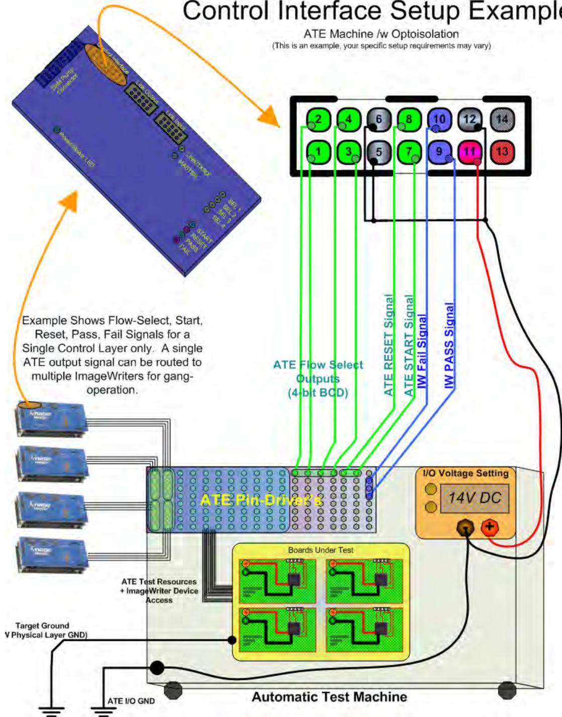
Figure 7-9—Setup Example for Control Interface to ATE
