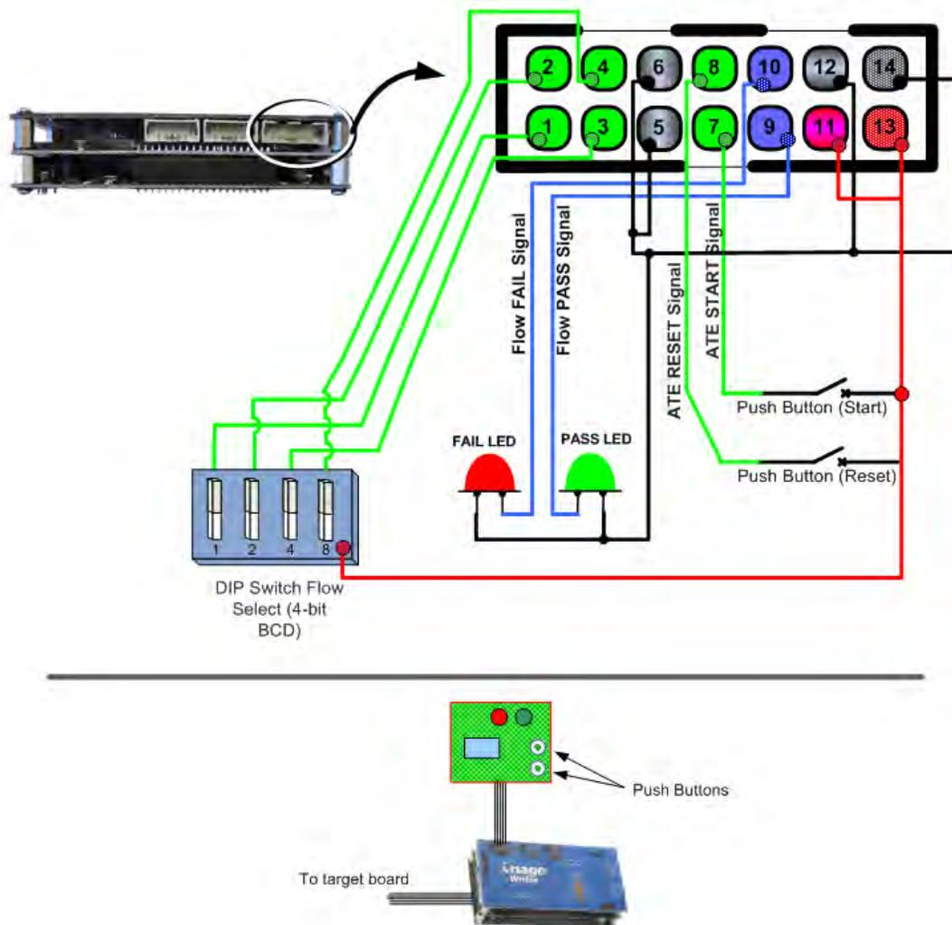
Figure 2-9—Push Button **Without** Isolation
