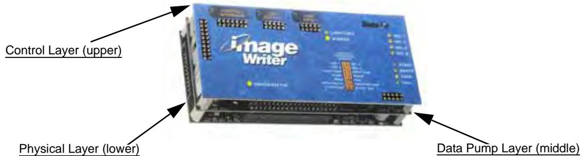
Figure 1-5—IW-300 Showing Three Layers of Hardware
