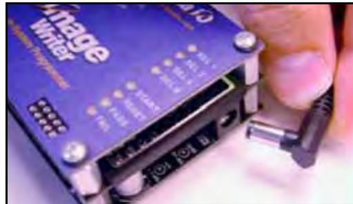
Figure 2-2—Plug AC Adapter into Auxiliary Power Connector
