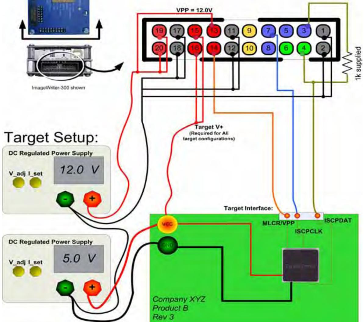
Figure 7-8—Setup Example for Microchip Serial Protocol
