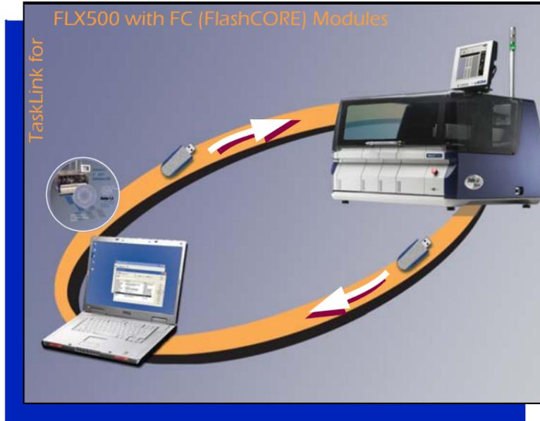
The Data I/O FLX500 is a desktop solution for production programming and handling of semiconductor devices (NAND and NOR, Micros, Serial, SD Cards, etc.).
