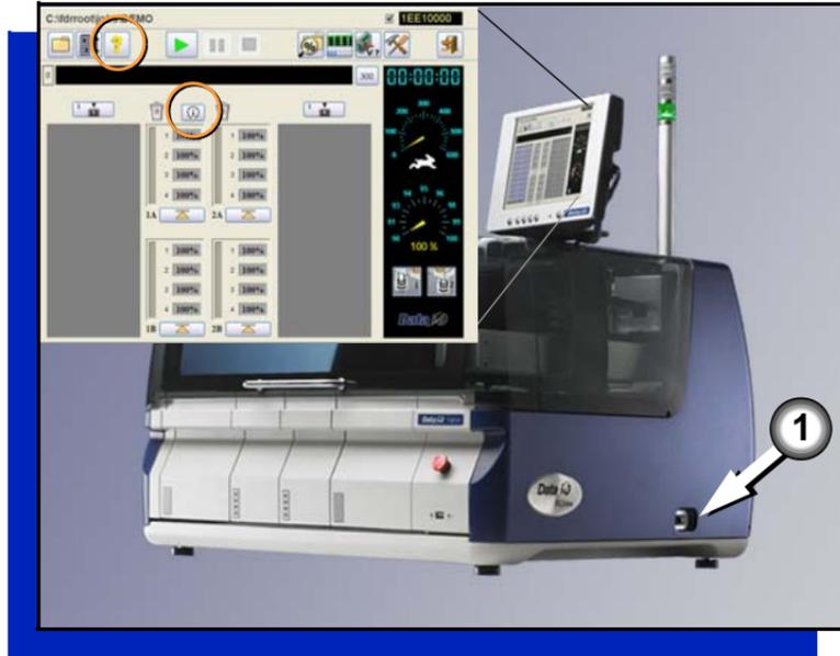
Power can be switched On without modules or Socket Adapters installed.
