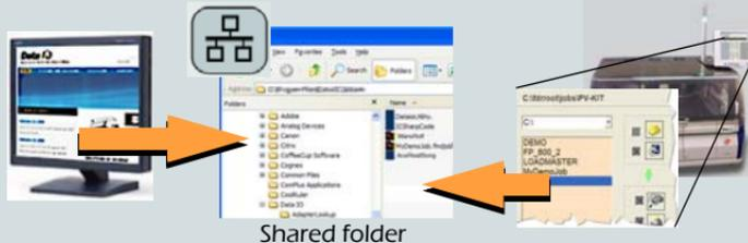
The Job Window can be set up to show jobs in the FLX C: drive [1] by sharing the FLX host computer, or in a network shared directory [2] by mapping n:\fdrrroot\ folder on a PC (with TaskLink). Use standard Windows procedures for network connections.
