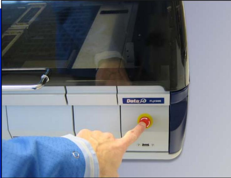
Pushing the Emergency Stop will stop the gantry immediately. It does not clear devices/cards from the programmers.
