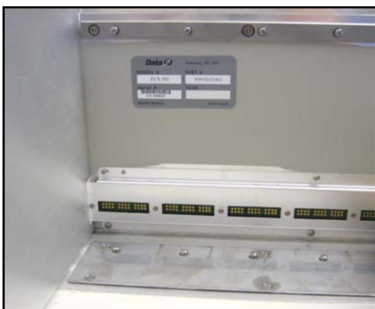
Figure 18—The Serial Number Label is visible after removing the modules.
