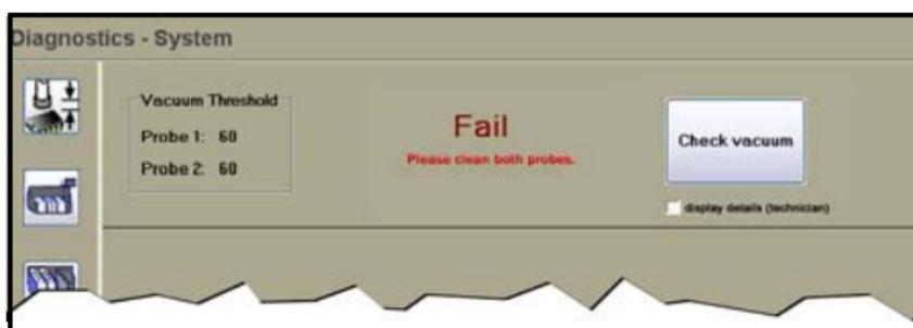
Figure 10—The Check Vacuum button on the System Window in the Diagnostics Tools and the Fail message when the system does not meet requirements.
