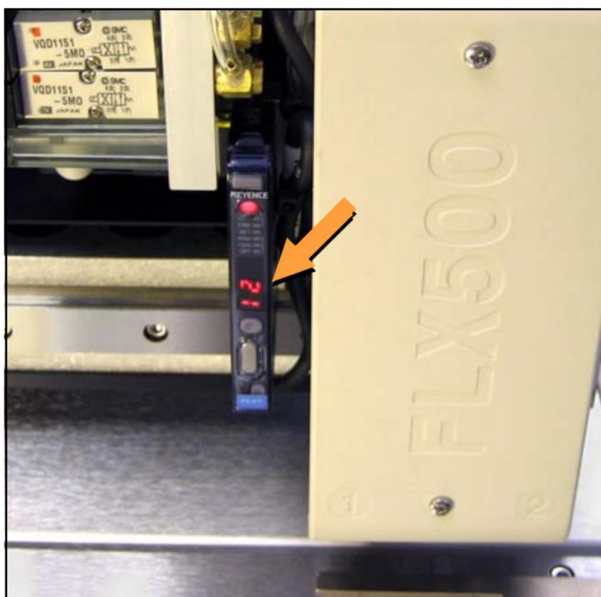
Figure 16—PNP Head optic sensor digital display showing a reading of 12.
