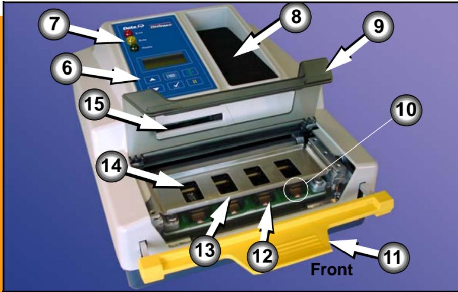
6. Control Panel with LCD display
