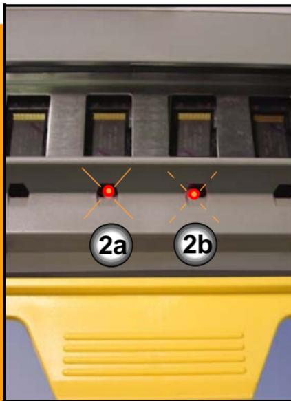
2. ● Red lamp = At least one device in the current block failed to program.
