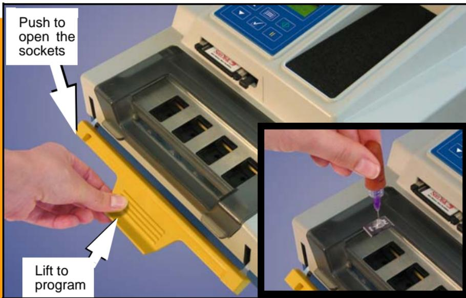
To run a job (with Auto Start on) push the Actuating Bar down, load the sockets, lift the Bar to program. When the yellow lamp stops blinking, push the Bar down and remove devices. Continue until the job is done.
