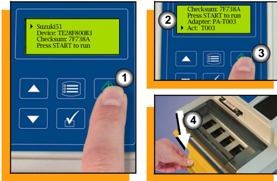
FlashPAK II has the option to load source data from a master device rather than a computer file.
