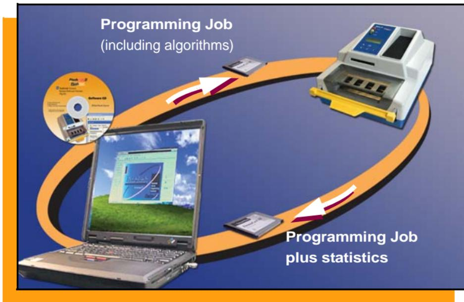
Data I/O's FlashPAK II is a scalable solution for engineering and manual production programming of Flash memory devices, many microcontrollers, and EPROMs. TaskLink™ for FlashPAK II™ (included) is software required to create and manage jobs. A job is all the information required to program devices.
