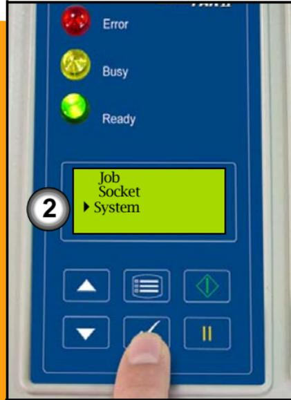
Auto Start is the feature which allows FlashPAK II to begin programming simply by lifting the Actuating Bar (it also closes the sockets). When Auto Start is disabled, you must press Start after closing the sockets to begin programming each block of devices.
