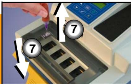
5. Put your master device into any socket. Ensure that the other three sockets are empty.
