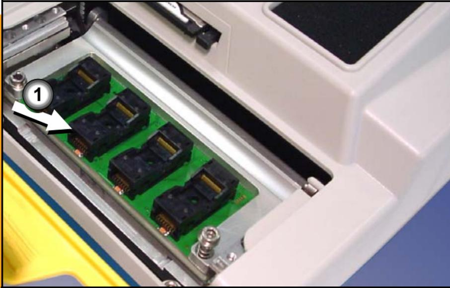
Use compressed air to prevent dust accumulation in the sockets.
