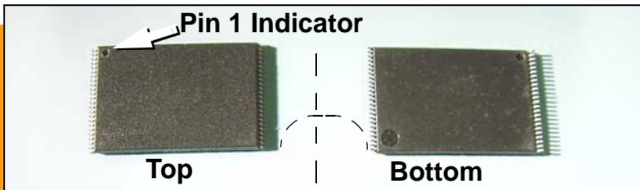
Most devices have a dimple located at pin 1. See manufacturers' specifications.
