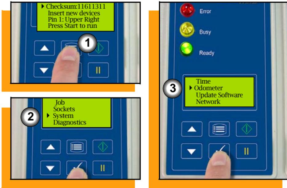
The odometer displays the total hours that FlashPAK II has been switched on, and total devices that **PASSED** programming. These settings cannot be altered.
