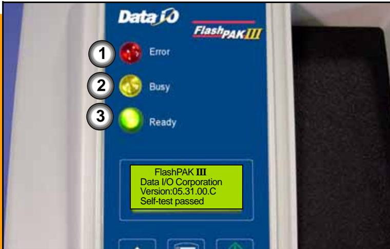
1. **Red** - One or more devices currently loaded has failed programming; or the Self-test failed; or any other errors.
