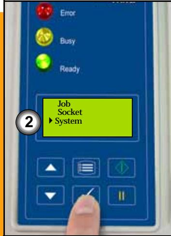
Auto Start is the feature which allows FlashPAK to begin programming simply by lifting the Actuating Bar (it also closes the sockets). When Auto Start is disabled, you must press Start after closing the sockets to begin programming each block of devices.
