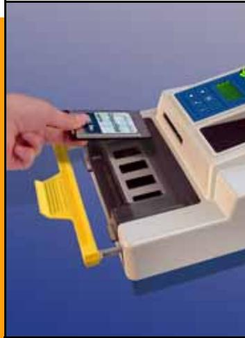
Periodically, updates to FlashPAK III's system software will be available. An update is loaded from a PC card.
