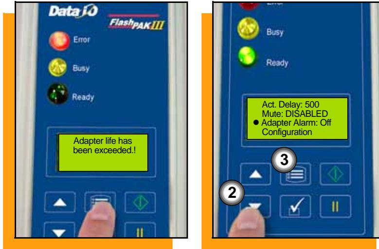
The Socket Life Exceeded message appears when the Sockets have been actuated a recommended number of cycles (see Socket > Adapter Statistics > Adapter Life.)
