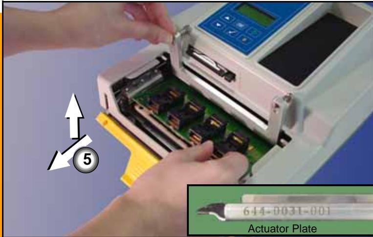
5. Without touching the gold contact surfaces on the bottom of the Socket Adapter, lift it up off the dowel pins, and out.
