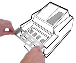
**NOTE:** The yellow Actuating Bar must be in the up position.
