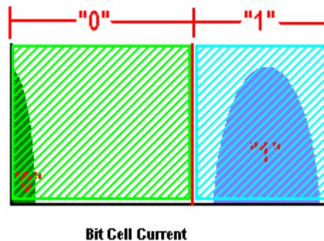
Figure 4. Testing for Under-Erased Cells
